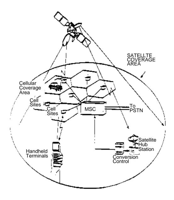
Figure 18. Hybrid Cellular Satellite Network
