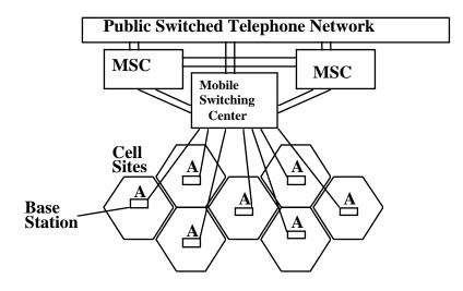
Figure 1. Cellular System Structure
