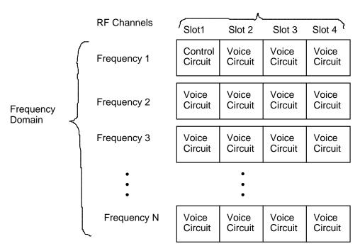
Figure 5. TDMA Cellular System Architecture
