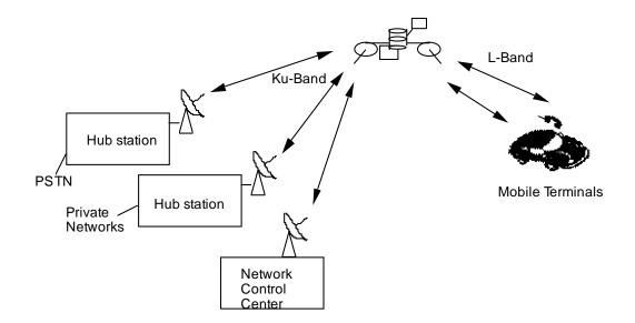
**Figure 17. Mobile Satellite Network**
