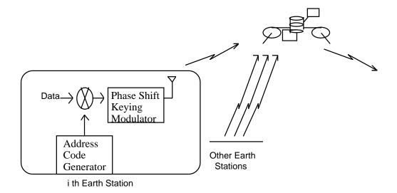
Figure 16. CDMA Satellite System Architecture
