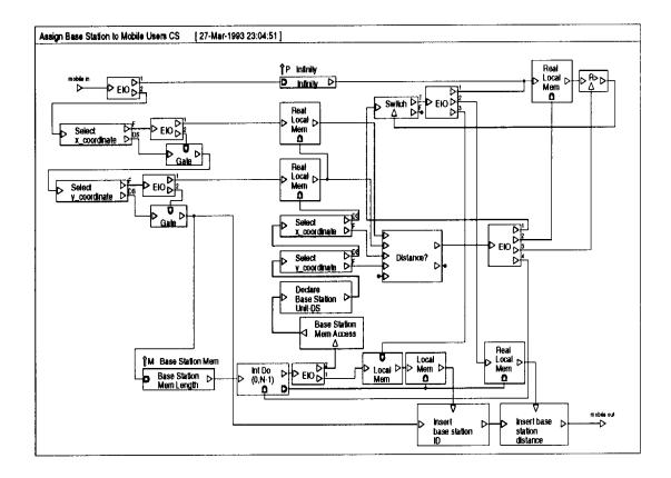
Figure 28. Assign Base Station to Mobile User CS
