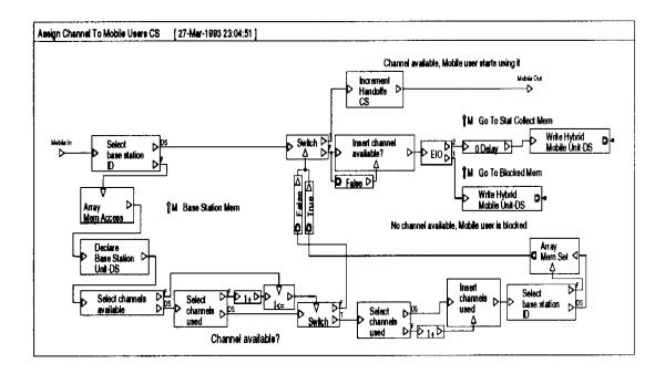
Figure 29. Assign Channel to Mobile User CS
