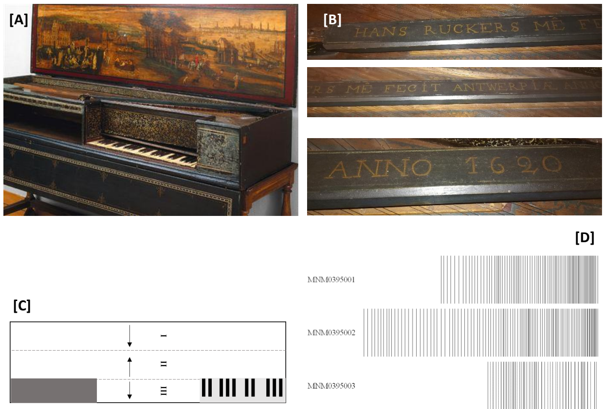
Figure 13. [A] Dutch virginal (MNM0395, MNM), assigned to Hans Ruckers family, from XVI/XVII century (Photo credits: ©José Pessoa/DGPC-ADF); [B] inscriptions “HANS RUCKERS MÊ FECIT ANTWERPIAE ANNO 1620” (Photo credits: ©Alexandra Lauw/CEF-ISA); [C] Layout of the boards on the soundboard [the arrow indicates the growth direction]; and [D] Grid beam graph representing the tree ring widths of each board.
