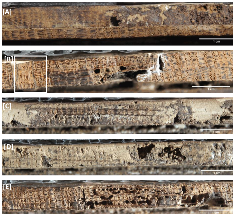
Figure 33. Transverse sections of oak boards from Mater Misericordiae , NMCPMS, assigned to Portuguese painter Gregório Lopes: [A] with and without preparation; [B] newer wood; [C] consolidation plaster; [D] wood degradation; and [E] xylophagous galleries (SOURCE: CEF-ISA unpublished).
