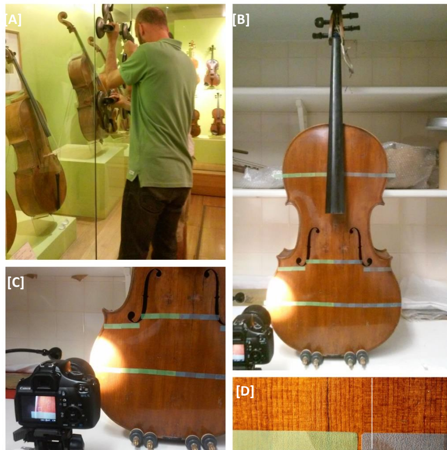
Figure 36. Dendrochronological study stages of a Portuguese cello, MNM, assigned to Joaquim José Galvão: [A] window removal; [B] cello without strings and labelling in three levels for the growth rings measurements; [C] radial cross-section macro-photographs; and [D] separation between bass side and treble side.
