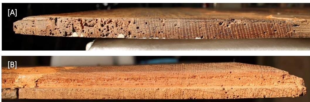
Figure 56. [A] Overview of the board I with the original thickness in Encontro de Abraão e Melquisedeque (93 Pint); and [B] Overview of the board II with bevelled edges in São Boaventura e São Luís de Tolosa (99 Pint).
