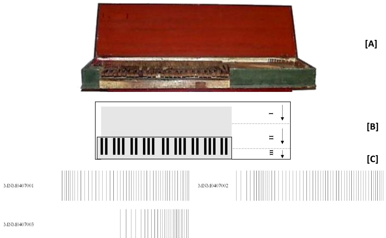
Figure 2. [A] Portuguese clavichord (MNM0407, MNM), unknown attribution, from 1750-1790 (SOURCE: MatrizNet); [B] Layout of the boards on the soundboard [the arrow indicates the growth direction]; and [C] Grid beam graph representing the tree ring widths of each board.
