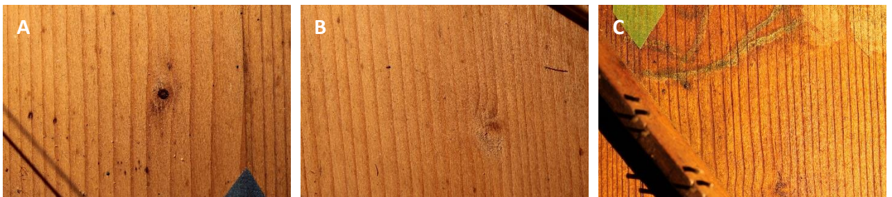
Figure 80. Knots in: [A-B] board V and VII in the Portuguese harpsichord (MNM0681) of unknown attribution; and [C] board IV in the Dutch harpsichord (MNM0374) of unknown attribution.
