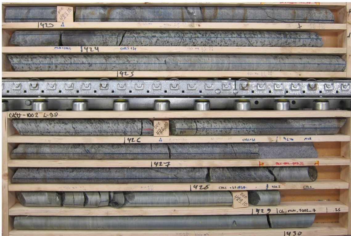
Figure 13. Variable mafic rocks within one sill/dyke. From 426.4 to 428.2 meters metagabbroic texture. On top of that, light green chlorite schist with biotite stacks that look like amphiboles. From 428.2 onwards, only silky, light green pure chlorite schist. Hole OKU-1002 from Kylylahti syncline's western limb. Core diameter 50.6mm.
