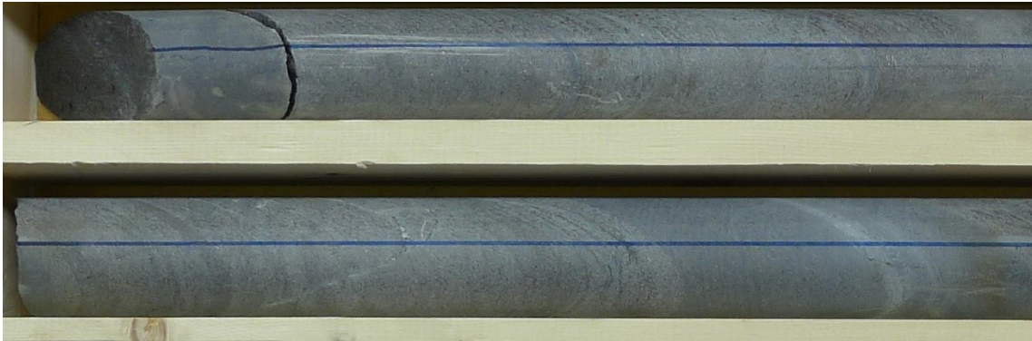
Figure 4. Typical mica schist of Kylylahti showing compositional banding and varying grainsize of micas. Core diameter 57.5mm.
