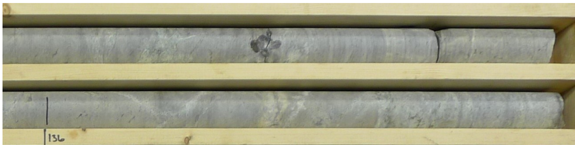
Figure 10. Outokumpu Alteration Assemblage carbonate rock. Tiny slightly elongated black specks are chromite crystals. Veinlets of coarser carbonate, usually calcite, cross-cutting through the dolomite-calcite-tremolite matrix. The amount of carbonate minerals greatly exceeds the amount of tremolite. Lighting conditions tilt the colour slightly towards yellow when compared to daylight. Hole KU-656, core diameter 40.7mm.
