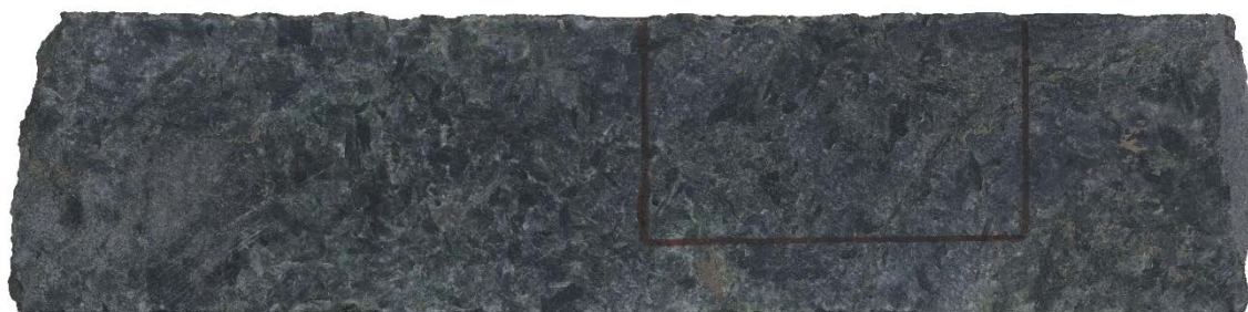
Figure 21. OME-Actska with coarse dark and green amphiboles, carbonates, and pyrrhotite with minor pentlandite and chalcopyrite. Sample KU-934-90,34. Note the typical bluish tint of the rock. Core diameter 40.7 mm.
