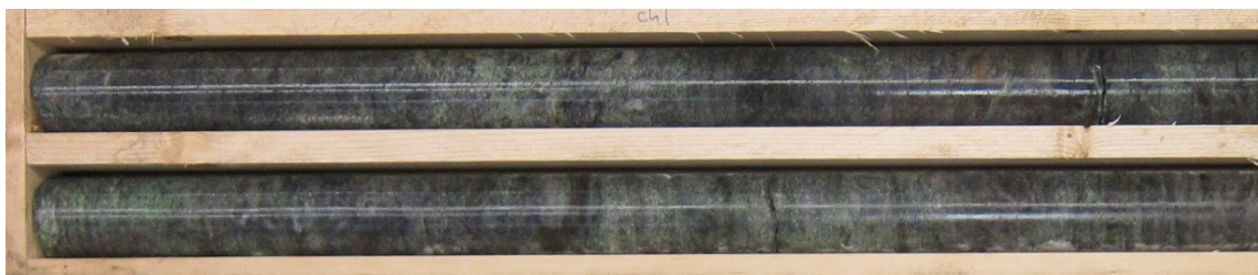
Figure 11. Picture of wet, unmineralized tremolite skarn from hole KU-656. Green Cr-tremolite, dolomite, calcite, and some quartz. Core diameter 40.7 mm.
