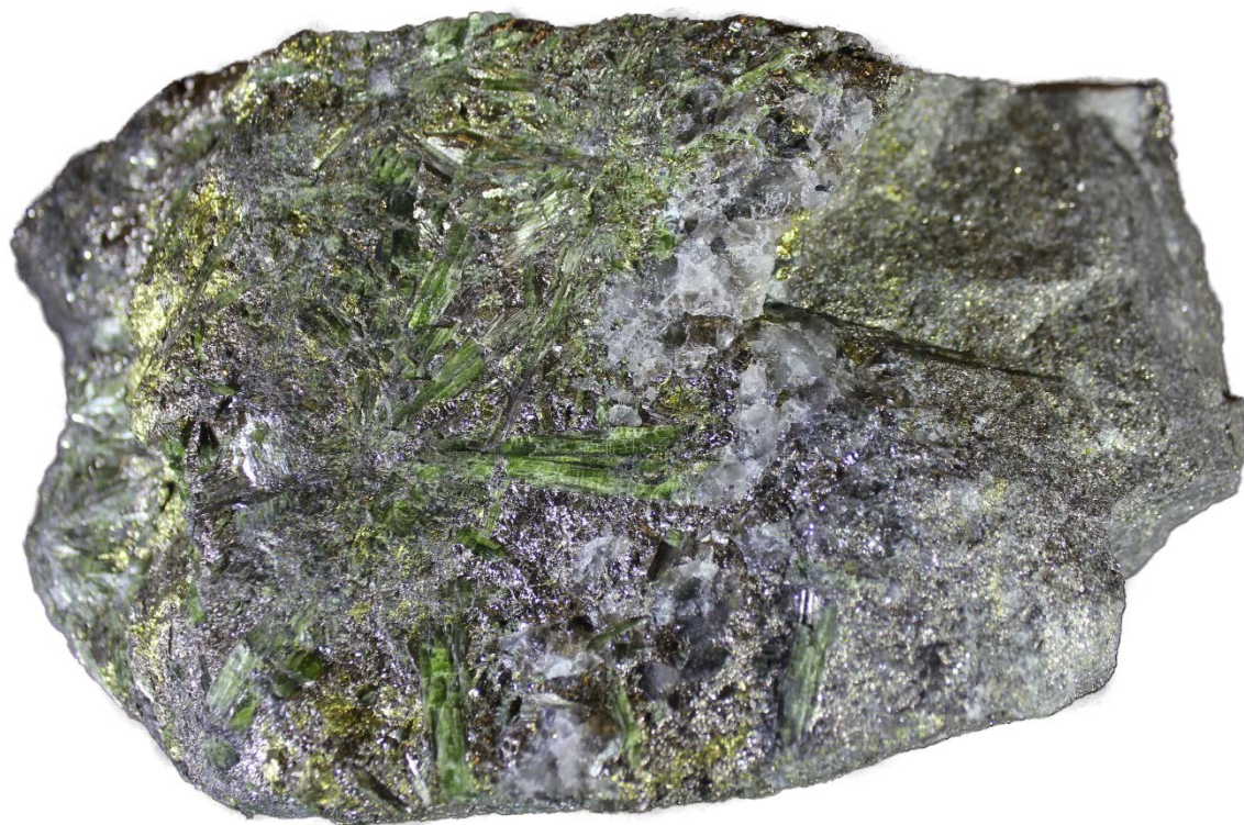
Figure 16. Disseminated ore in tremolite skarn from Kylylahti mine. Ore minerals include chalcopyrite, pentlandite and linnaeite-polydymite. Main gangue minerals are coarse Cr-tremolite, quartz, pyrrhotite, pyrite, dolomite, calcite and phlogopite. Sample is unanalysed, but based on its appearance, this is a rich disseminated ore with high grades of Cu, Ni, Co, and most likely Au. Sample width is 24cm. Sample collected by Mathias Backman from unknown location at Kylylahti mine.
