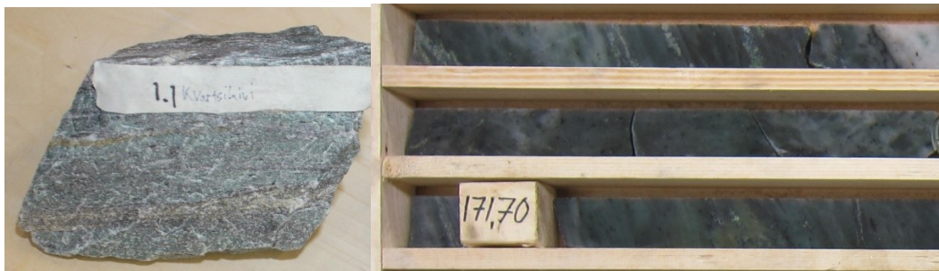
Figure 12. Left: Banded quartz rock of Kylylahti. Quartz, turquoise fine fuchsite, and not so common brown band that is most likely titanite and rutile or iron oxides, as is observed in similar Kylylahti quartz rock samples. Small, blackish specs are slightly elongated chromite crystals. Tape width is 26 mm. This sample nowadays belongs to Outokumpu Mining Museum collection. Right: Same minerals from drillhole KU-933. Core diameter 40.7mm.
