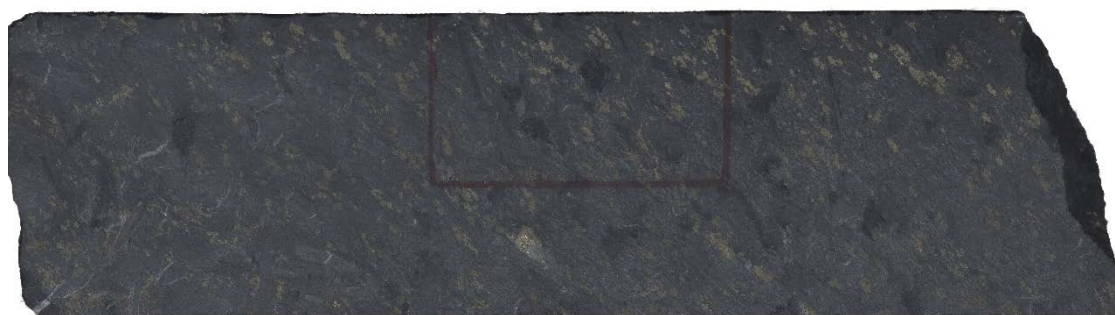
Figure 20. CRB-Actska carbonate rock sample OKU-1000-253,42 with dark, coarse amphiboles, pyrite, and graphite in dark carbonate rock. Core diameter is 50.6 mm. Red marker shows area where thin section will be made.
