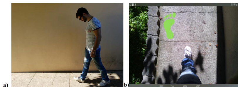
Figure 1. a) Photography displaying the HS event b) detection of the right heel-strike by ORA-2, and consequently display of the left footprint.
