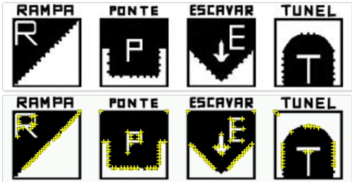
Figure 66: The initial design for the action markers after being redesigned for better detection with good features.
