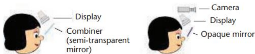
Figure 8: Difference between Optical (left) and Video (right) types of Head-Worn Displays. (Retrieved from Azuma et al. (2001))
