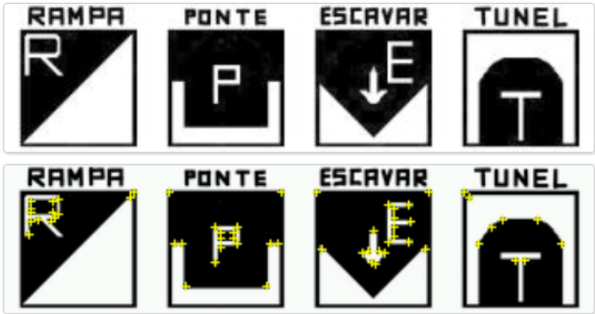
Figure 65: The initial design for the action markers did not generate enough features for good detection.
