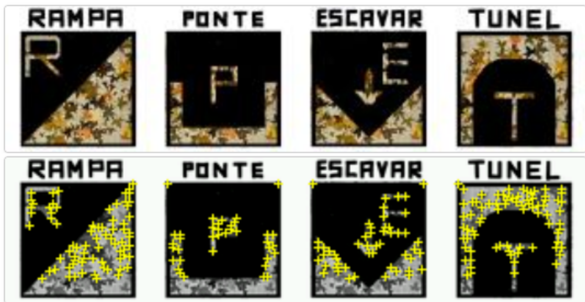
Figure 67: The addition of patterned backgrounds improved the features and allowed for better detection over conditions with poor light.
