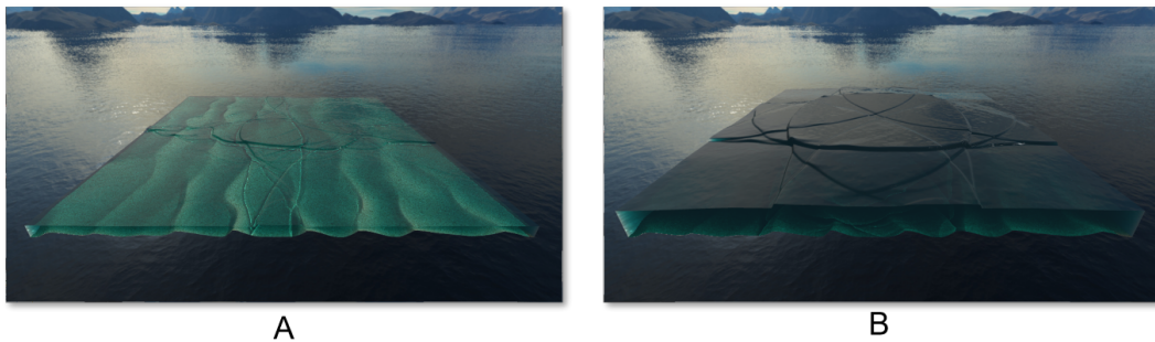
Figure 55: Scenes with different starting conditions but all other parameters equal. The scene on the right (B) has a higher average depth which results in faster waves.
