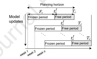
Figure 2: Rolling MRP planning horizon strategy with frozen and free periods for a component c.
