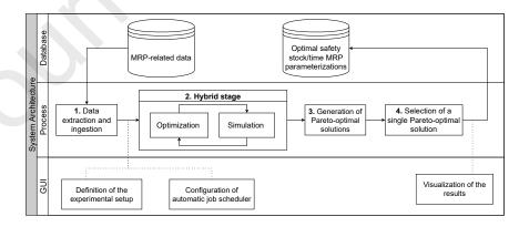
Figure 3: The system architecture of the proposed DSS.
