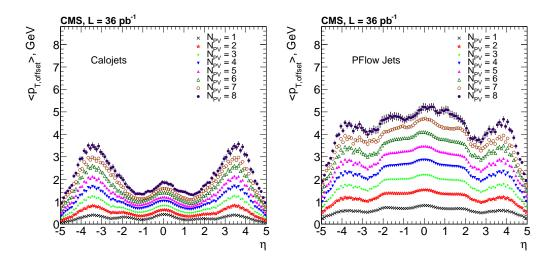
**Figure 2.** Average offset in  $p_T$ , as a function of  $\eta$ , measured in minimum bias events for different pile-up conditions (categorized according to the number  $N_{PV}$  of reconstructed primary vertices). Left: CALO jets. Right: PF jets.
