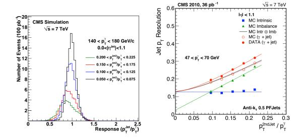
**Figure 36**. Response distributions in different bins of  $p_T^{\text{Jet2}}/p_T^{\gamma}$ , and for  $140 < p_T^{\gamma} < 180 \,\text{GeV}$  (left), components of the jet  $p_T$  resolution, as a function of  $p_T^{\text{Jet2}}/p_T^{\gamma}$  for PF jets in data and MC samples (right).
