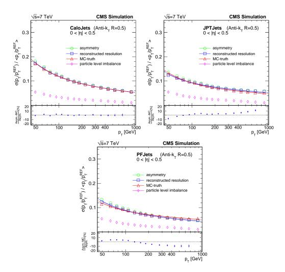
**Figure 32**. Application of the asymmetry method to simulated CALO (top left), JPT (top right), and PF jets (bottom) in  $|\eta| < 0.5$ . The reconstruction-level (green circle) and particle-level (magenta diamond) results are shown together with the final measurement (blue square), compared to the generator-level MC (denoted as MC-truth) derived resolution (red triangle).
