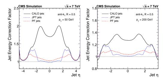
**Figure 6**. Monte Carlo jet-energy-correction factors for the different jet types, as a function of jet  $\eta$ . Left: correction factor required to get a corrected jet  $p_T = 50 \,\text{GeV}$ . Right: correction factor required to get a corrected jet  $p_T = 200 \,\text{GeV}$ .
