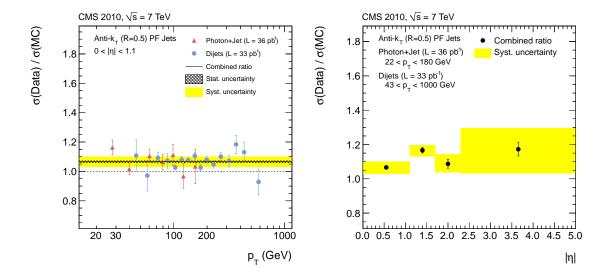
**Figure 39**. The ratio of jet  $p_T$  resolutions in data and MC samples vs.  $p_T$ , in  $|\eta| < 1.1$ , from dijet and  $\gamma$ +jet samples; a combination fit to both data sets is also shown (left). Results from the combination fits vs.  $p_T$  in various  $\eta$  ranges (right).
