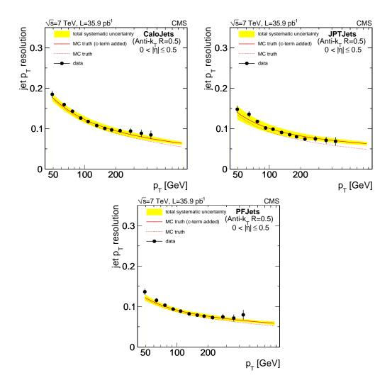
**Figure 34.** Bias-corrected data measurements, compared to the generator-level MC (denoted as MC-truth)  $p_T$  resolution before (red-dashed line) and after correction for the measured discrepancy between data and simulation (red-solid line) for CALO (top left), JPT (top right), and PF jets (bottom) in  $|\eta| < 0.5$ .
