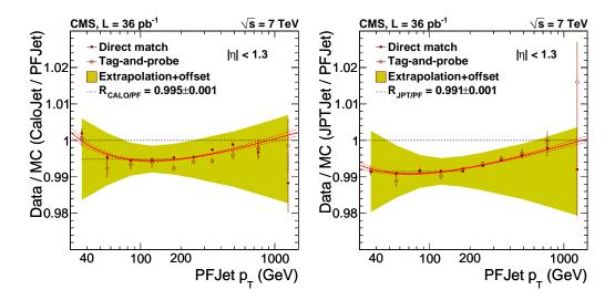
**Figure 24.** Left: CALO vs. PF jet  $p_T$  response ratio between data and MC simulation. Right: JPT vs. PF jet  $p_T$  response ratio between data and MC simulation. The solid circles correspond to direct matching in the  $\eta - \phi$  space and the open circles correspond to a tag (PF jet) and probe (CALO/JPT jet) method.
