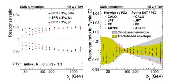
**Figure 21**. Left: sensitivity of the jet energy response in  $|\eta| < 1.3$  to the single-particle response (SPR) uncertainty. Right: dependence of the jet energy response on the fragmentation model. Here AK7PF stands for PF jets reconstructed with the anti- $k_T$  algorithm with size parameter R = 0.7.
