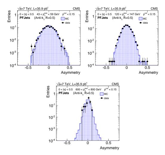
**Figure 31**. Examples of PF jet asymmetry distributions for  $|\eta| < 0.5$  and a low- $p_T^{\text{ave}}$  bin (top left), a medium- $p_T^{\text{ave}}$  bin (top right) and a high- $p_T^{\text{ave}}$  bin (bottom), determined from QCD simulation (blue histograms) and compared with the result from data (black dots).
