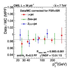
**Figure 19**. Ratio of data over MC for the MPF response, as a function of  $p_T^{\gamma,Z}$  in the photon+jet sample (circles),  $Z(e^+e^-)$ +jet sample (triangles) and  $Z(\mu^+\mu^-)$ +jet sample (squares).
