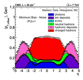
**Figure 3**. Breakdown of the average offset  $p_T$ , in terms of the PF candidates, as a function of  $\eta$ , for events with one PU interaction. Data are shown by markers and MC is shown as filled histograms.
