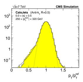
**Figure 29**. Distribution of the simulated CALO jet response,  $p_T^{\text{reco}}/p_T^{\text{gen}}$ , in a particular  $|\eta|$  and  $p_T^{\text{gen}}$  range. Fit examples with a Gaussian and a double-sided Crystal-Ball function are shown.
