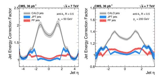
**Figure 26**. Total jet-energy-correction factor, as a function of jet  $\eta$  for  $p_T = 50 \,\text{GeV}$  (left) and  $p_T = 200 \,\text{GeV}$  (right). The bands indicate the corresponding uncertainty.
