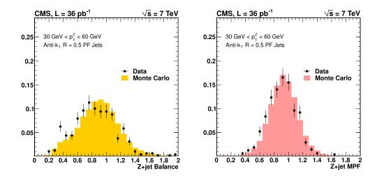
**Figure 18**. Left: jet energy response from  $Z(\mu^+\mu^-)$ +jets  $p_T$ -balancing in the bin  $30 < p_T^Z < 60 \,\text{GeV}$ . Right: jet energy response from  $Z(\mu^+\mu^-)$ +jets MPF in the bin  $30 < p_T^Z < 60 \,\text{GeV}$ .
