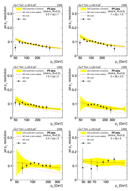
**Figure 35**. Bias-corrected data measurements, compared to the generator-level MC (denoted as MC-truth) resolution before (red-dashed line) and after correction for the measured discrepancy between data and simulation (red-solid line), compared to data, for PF jets in different  $\eta$  ranges.
