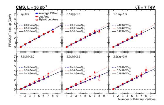
**Figure 4**. Average PF jet pile-up  $p_T$ , as a function of the number of reconstructed vertices ( $N_{PV}$ ) for the jet area, the average offset, and the hybrid jet area methods in 6 different  $\eta$  regions. In the y-axis title, PFAK5 denotes the PF jets reconstructed with the anti- $k_T$  algorithm with distance parameter R = 0.5.
