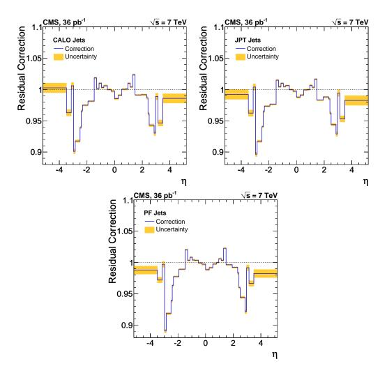
**Figure 13**. Relative jet energy residual correction as a function of jet  $\eta$  for CALO, JPT and PF jets respectively. The band shows the uncertainty due to statistics, radiation corrections, and asymmetry in  $\eta$ .
