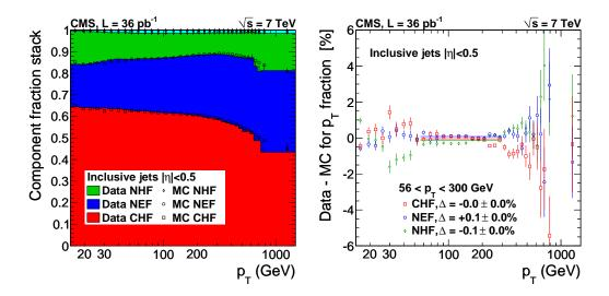
**Figure 23**. PF jet composition. Left: energy fraction carried by charged hadrons (CHF), photons (NEF), and neutral hadrons (NHF) as a function of jet  $p_T$  in the region  $|\eta| < 0.5$ . The filled histograms and the markers represent the data and the simulation respectively. Right:  $p_T$  fraction difference between data and MC.
