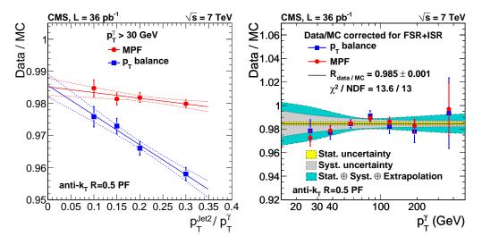
**Figure 17**. Left: dependence of the data/MC ratio of the jet energy response on the second jet  $p_T$  threshold. Right: data/MC ratio of the jet energy response, after extrapolation to zero second jet  $p_T$ , as a function of  $p_T^{\gamma}$ . Solid squares and solid circles correspond to the  $p_T$ -balancing and the MPF methods, respectively.
