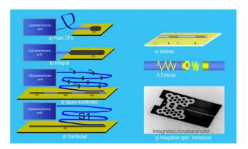
**Figure 6:** Illustration of photonic sensors according to the technology and the interaction of light-Oy-Mx: (a-f) Optical Fiber Sensors and (g) Integrated Optic Sensor. Courtesy of the author.
