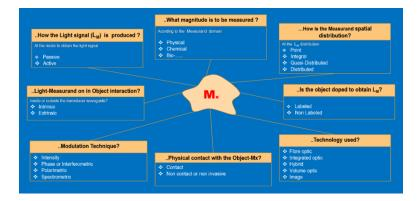
**Figure 5:** Types of photonic sensors taking into consideration aspects concerning the measurand (Mx) on/in the object (Oy) and the modulated Light (LM). Courtesy of the author.
