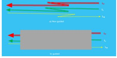
**Figure 2:** Illustration of the optical channel of a photonic sensor. According to the media used to transmit the Light to and from the object: (a) non guided optical channel and (b) waveguide optical channel (typically optical fiber cables). Courtesy of the author.
