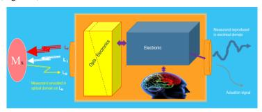
**Figure 3:** Illustration of the optoelectronic unit of a photonic sensor. It is in charge of producing and controlling the photonic beams or Light (if required) to carry out the object's interrogation or/and pumping tasks. It is also in charge of achieving the photodetection, and all required additional processes, to
