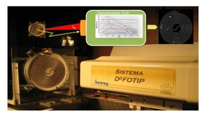
**Figure 12:** Illustration of SPA-IRT sensor device for online quality control of radiant heaters. After a short energy pulse, the infrared radiations of the cooling process of the heaters were captured and properly treated/processed with adequate algorithms; images with detected defects were synthesized and the OU's output offered actuation signals. Made by the author based on material courtesy of Photonics Engineering Group of the University of Cantabria, UC.
