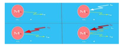
**Figure 1:** The focus at the measurand on/in the object illustrates main sensing possibilities using light techniques. Light modulated by the measurand  $(L_M)$  on/in the object: (a) produced by the object itself; (b) returning from the object consequence of the interrogation light (Li); (c) produced as a consequence of a pumping light (Lp) and (d) produced as a consequence of a pumping and interrogation lights. Courtesy of the author.
