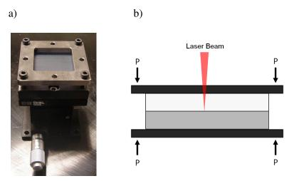
Figure 1. a) Experimental and b) schematic set-up for laser welding of ABS plates. Bottom part: ABS with additives (CNT), top part: ABS without filled.
