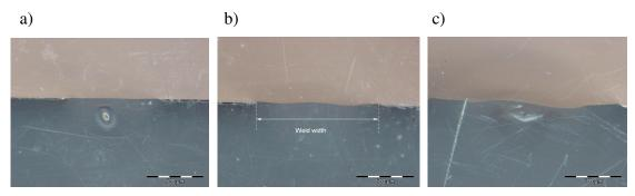
Figure 8. Optical micrographs of a representative a) poor joint P=6W b) optimal joint P=8.5W c) degraded joint done with P=16.5W in the case of ABS/ABS-0.01%CNT at v=15mm/s.
