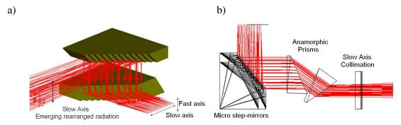
Figure 2. a) Realization of beam rearranging by a pair of step-mirrors consisting of 13 steps. b) Top side view of the compression unit.
