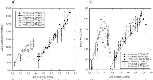
Figure 9. Average a) weld width b) shear force as a function of line energy for two different percentages of CNTs.
