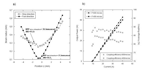
Figure 7. a) Beam quality measurement of the laser system at 6W of laser power emission; b) Output power and coupling efficiency for a  $600\mu m$  and  $400\mu m$  fibers both with numerical aperture of 0.22.
