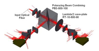
Figure 3. Ray tracing of the arrangement of two JOLD-50-CPBN-1L fiber coupling.
