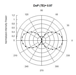
Figure 4. Polarization plot of a JOLD-50-CPBN-1L at 5W of laser power emission.
