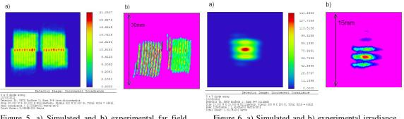
Figure 5. a) Simulated and b) experimental far field irradiance of the reshape laser beam after the micro-step mirrors at 10W of laser power emission. Vertical: Slow Axis, Horizontal: Fast axis.
