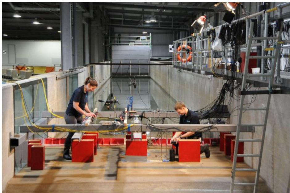
Figure 6. HR Wallingford's Froude Modelling Hall. The picture shows the 4m wide Fast Flow Facility during tests conducted for URBANWAVES, with the Tsunami Simulator seen at the far end of the flume.
