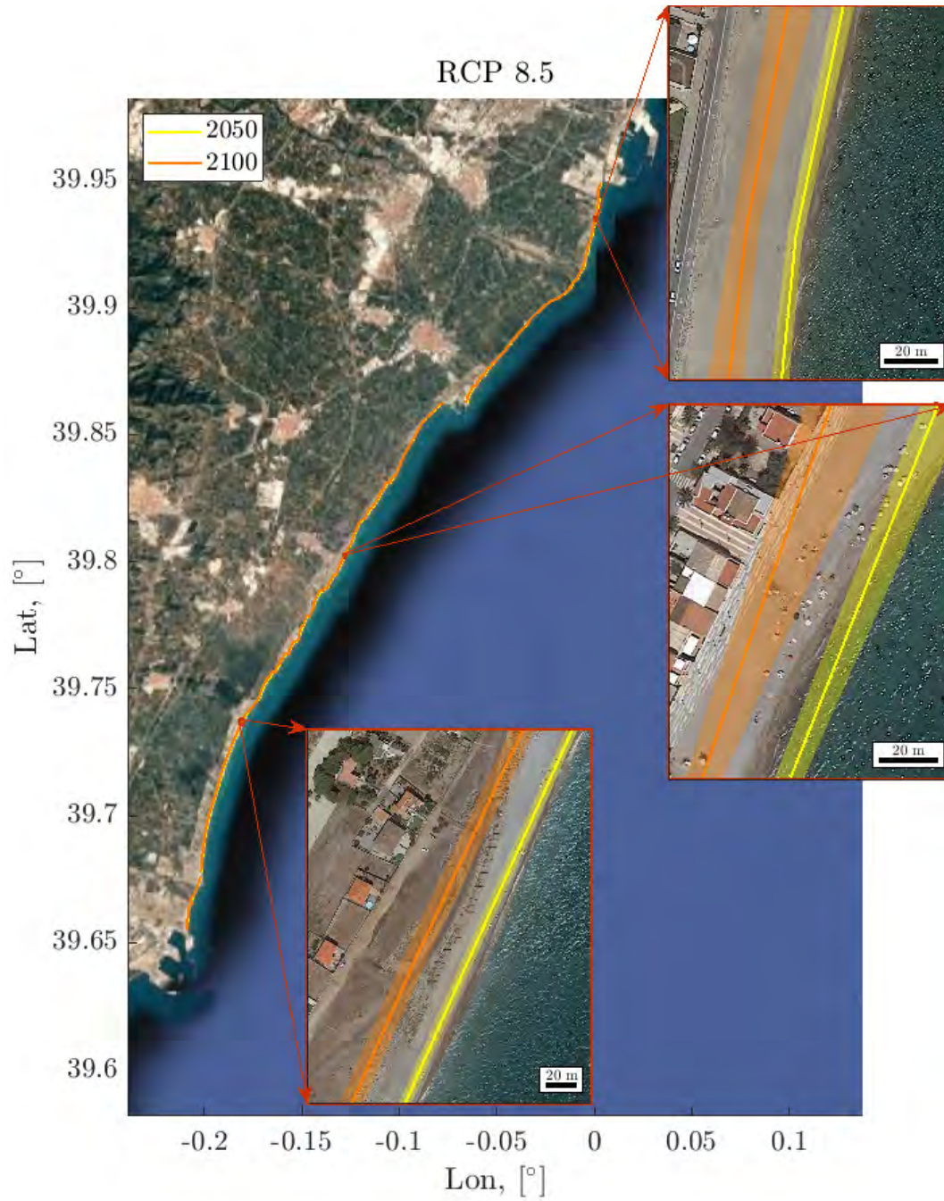
Figure 3.9: Tourist season shorelines (May, June, July, August, September) for 2050 and 2100 in Torre (top panel), Moncófar (middle panel) and Almenara (lower panel). Solid lines represent the median and the bands correspond to the 50% confidence interval of the 15 RCM and SLR percentile configuration for the RCP8.5.
