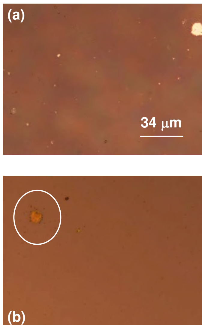
Figure 5.3: Optical microscope images showing visible deterioration of \text{Pr}_{2-x}\text{Ce}_x\text{CuO}_{4\pm\delta} thin films. (a) Example of “pinholes” which develop during film growth (sample JP15-17). The pinholes are the small white spots scattered around the viewing area. (b) Example of decomposition circled in white (sample JP19-17). The light tan colored spot (inside the white circle) is surrounded by black pepper looking spots. The black pepper spots are also seen without the light tan spot, but with much less frequency.
