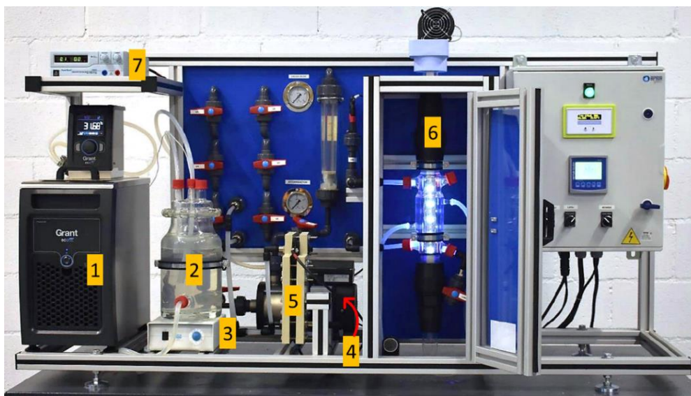
Figure 2.2. Experimental set-up used in the electrochemical oxidation experiments (APRIA Systems., S.L.).
