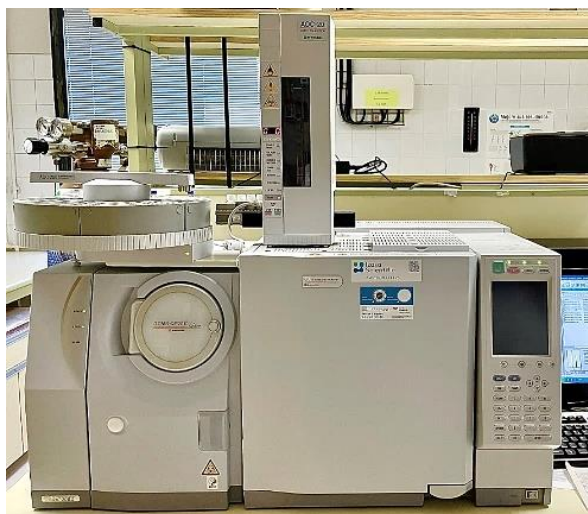
Figure 2.6. GC-MS Shimadzu QP2010 equipped with an auto-injector AOC-20i employed in the intermediate compounds analysis.
