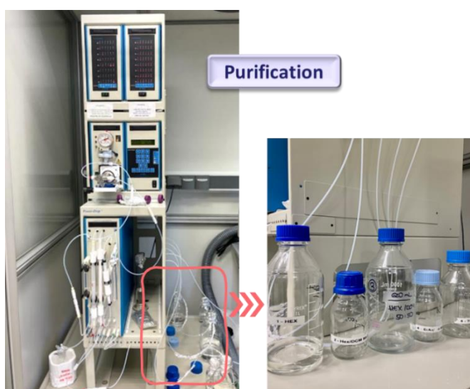
Figure 2.13. Automated clean-up system (Power-Prep™, Fluid Management Systems Inc., Waltham).
