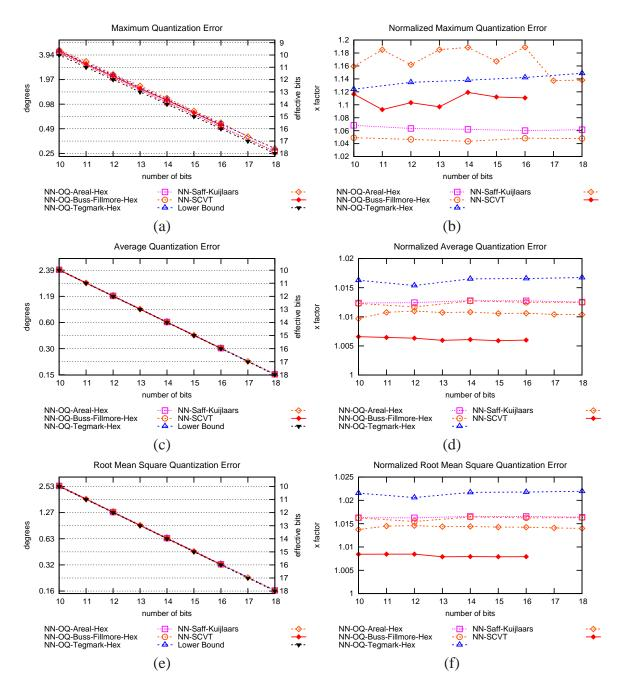
Figure 3.17: Different error statistics of the NN-OQ-Gnomonic-Hex, the NN-OQ-Areal-Hex, the NN-OQ-Buss-Fillmore, the NN-OQ-Tegmark, the NN-Saff-Kuijlaars, and the NN-SCVT quantization methods. (a,b) Maximum Quantization Error. (c,d) Average Quantization Error. (e,f) Root Mean Square Quantization Error.
