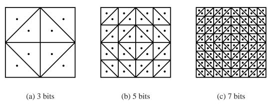
Figure 3.4: Pattern of representative points for an odd number of bits.
