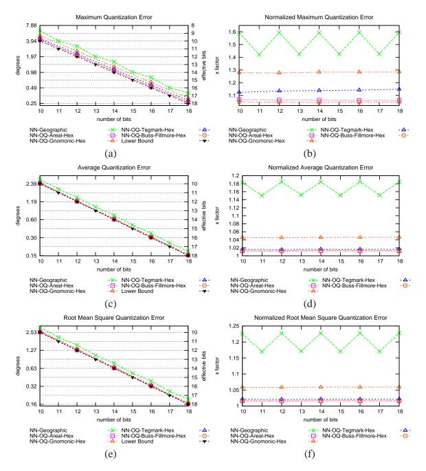
Figure 3.16: Different statistics of the NN-Deering, the NN-Geographic, the NN-OQ-Gnomonic-Hex, the NN-OQ-Areal-Hex, the NN-OQ-Buss-Fillmore-Hex, and the NN-OQ-Tegmark-Hex quantization methods. (a,b) Maximum Quantization Error. (c,d) Average Quantization Error. (e,f) Root Mean Square Quantization Error.
