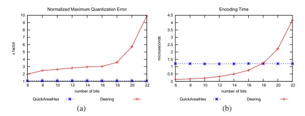
Figure 3.29: A comparison of the Deering and QuickArealHex methods. (a) Normalized Maximum Quantization Error. (b) Encoding time.
