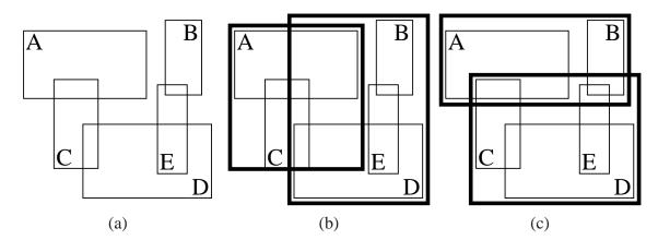
Figure 4.1: Arrangement of bounding boxes. (a) A set of five boxes. (b) One bounding box for boxes (A, C) and one for (B, D, E). (c) One bounding box for boxes (A, B) and one for (C, D, E).
