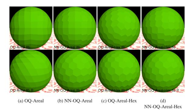
Figure 3.24: Rendering a perfect sphere with quantized normals at 8 bits, using the OQ-Areal, the NN-OQ-Areal, the OQ-Areal-Hex, and the NN-OQ-Areal-Hex quantization methods. The spheres in the top row have been rotated in the bottom row in order to show the tessellations from a different viewpoint.
