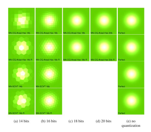
Figure 3.28, continued: Rendering the sphere in Figure 3.27(a) with surface normals quantized with 14, 16, 18, and 20 bits using the Deering, the OQ-Gnomonic-Hex, the NN-OQ-Areal-Hex, and the NN-SCVT quantization methods.
