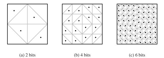
Figure 3.6: First step in constructing the hexagonal pattern for an even number of bits.
