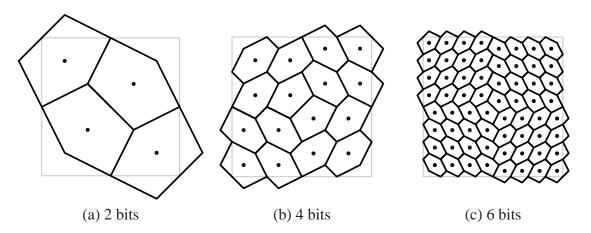
Figure 3.8: Hexagonal pattern of representative points for an even number of bits.
