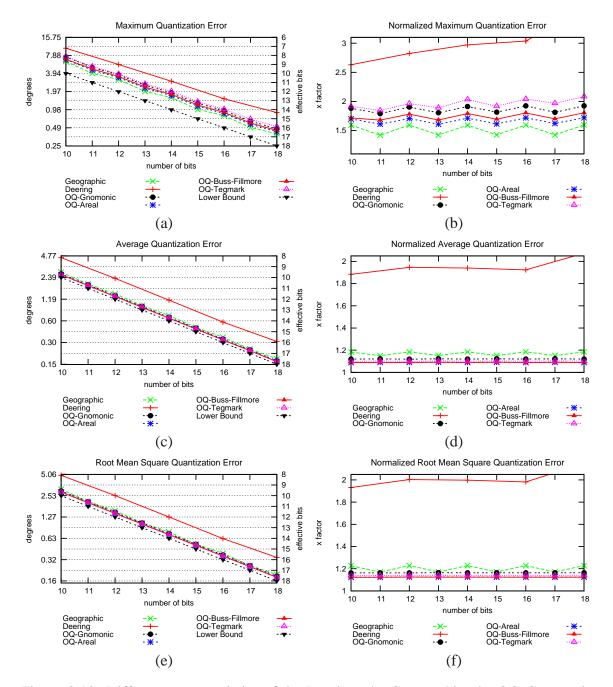
Figure 3.13: Different error statistics of the Deering, the Geographic, the OQ-Gnomonic, the OQ-Areal, the OQ-Buss-Fillmore, and the OQ-Tegmark quantization methods. (a,b) Maximum Quantization Error. (c,d) Average Quantization Error. (e,f) Root Mean Square Quantization Error.
