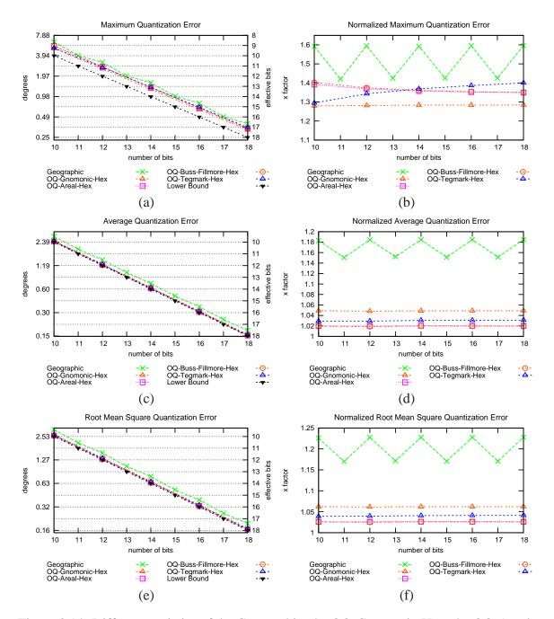
Figure 3.14: Different statistics of the Geographic, the OQ-Gnomonic-Hex, the OQ-Areal-Hex, the OQ-Buss-Fillmore-Hex, and the OQ-Tegmark-Hex quantization methods. (a,b) Maximum Quantization Error. (c,d) Average Quantization Error. (e,f) Root Mean Square Quantization Error.
