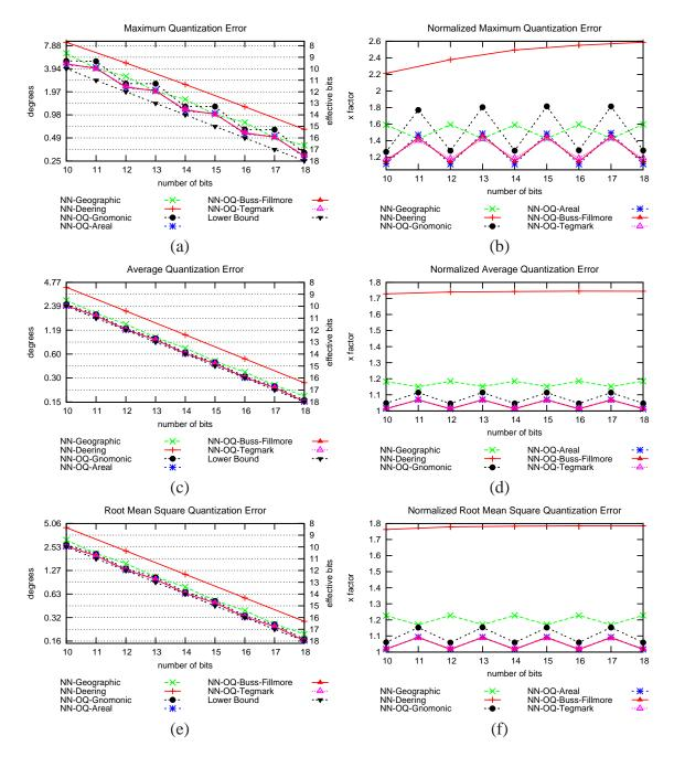
Figure 3.15: Different statistics of the NN-Deering, the NN-Geographic, the NN-OQ-Areal, the NN-OQ-Buss-Fillmore, and the NN-OQ-Tegmark, quantization methods. (a,b) Maximum Quantization Error. (c,d) Average Quantization Error. (e,f) Root Mean Square Quantization Error.
