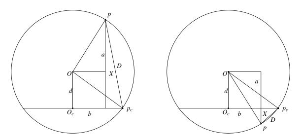
Figure 2.6: Finding the distance of a point to a circle.
