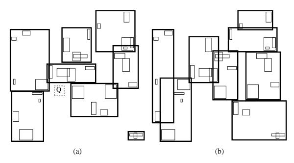
Figure 4.3: Result of applying the top-down packing TGS bulk loading algorithm to bulk load an R-tree using a cost function that minimizes (a) the overlap area, and (b) the total area.
