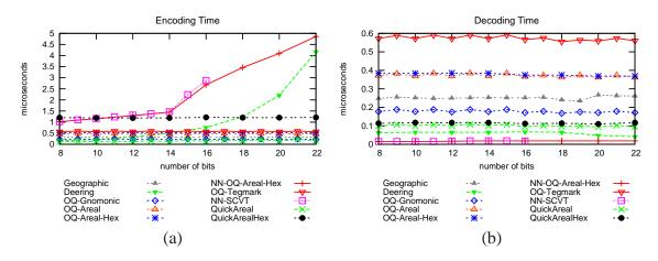
Figure 3.18: The quantization time of different quantization methods. (a) Encoding time. (b) Decoding time.
