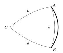
Figure 2.4: Excess of a spherical arc (shown in thicker line) between spherical points *A* and *B*. The thin lines are great circle arcs.
