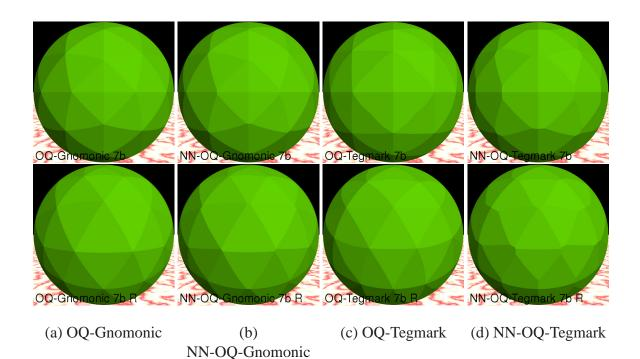
Figure 3.22: Rendering a perfect sphere with normals quantized with 7 bits, using OQ-Gnomonic, NN-OQ-Gnomonic, OQ-Tegmark, and NN-OQ-Tegmark quantization methods. The spheres in the top row have been rotated in the bottom row in order to show the tessellations from a different viewpoint.
