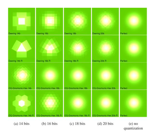
Figure 3.28: Rendering the sphere in Figure 3.27(a) with surface normals quantized with 14, 16, 18, and 20 bits using the Deering, the OQ-Gnomonic-Hex, the NN-OQ-Areal-Hex, and the NN-SCVT quantization methods.
