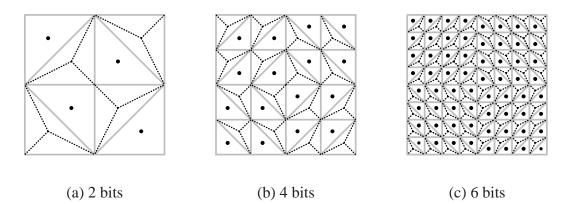
Figure 3.7: Second step in constructing the hexagonal pattern for an even number of bits.
