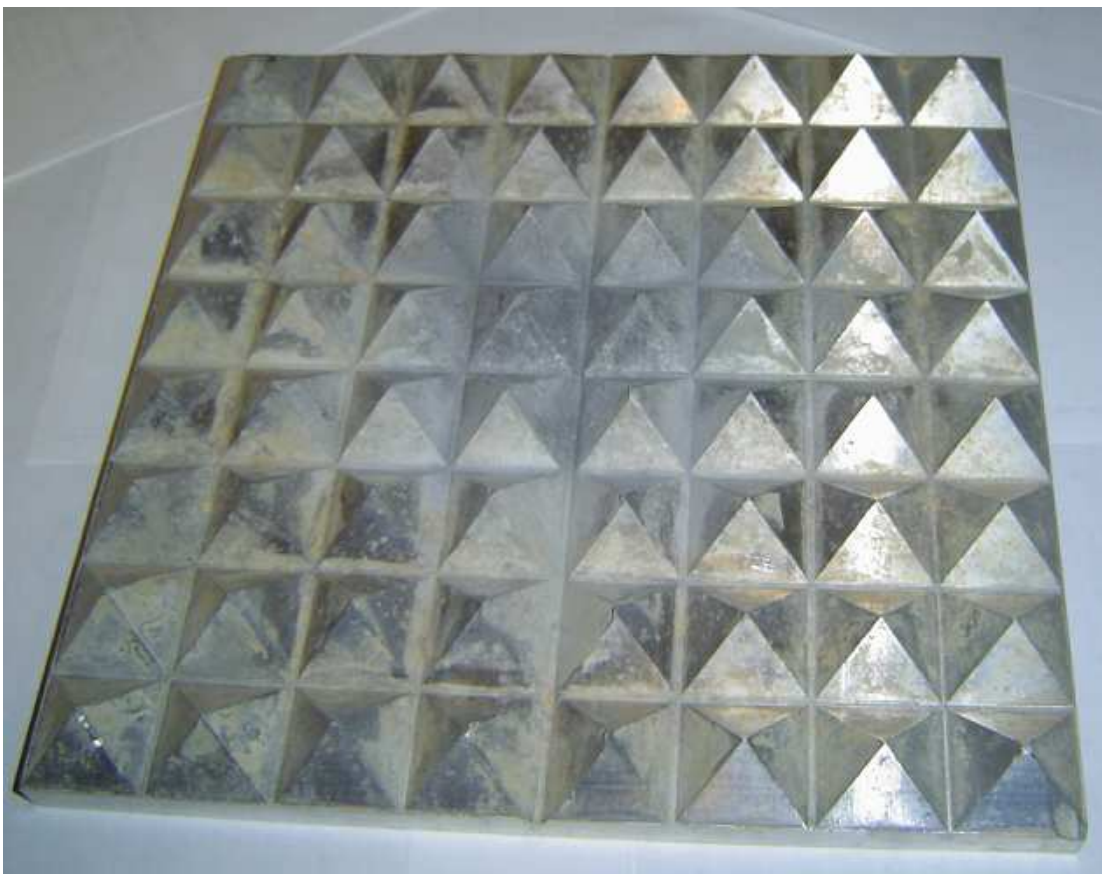
Figure B.5: Wear on 0.5” Pyramid Grid Plate After Testing
