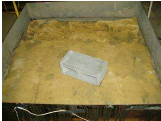
Figure 3.14: Compacted Sand Bed
