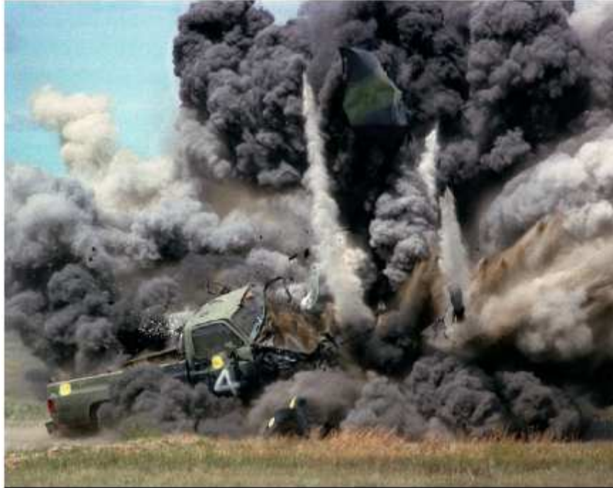
Figure 1.1: Unprotected 5/4 Ton Truck Against a 6.5kg TNT Antitank Mine [1]
