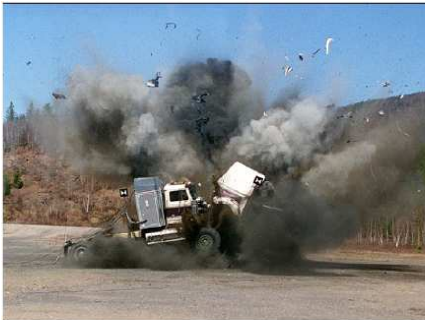
Figure 1.3: Fragments and Ejecta Created After Mine Blast [1]
