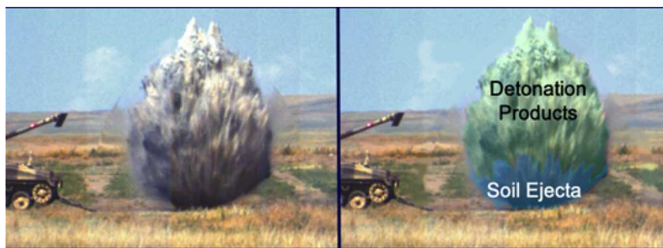
Figure 1.5: Detonation Products and Soil Ejecta [1]
