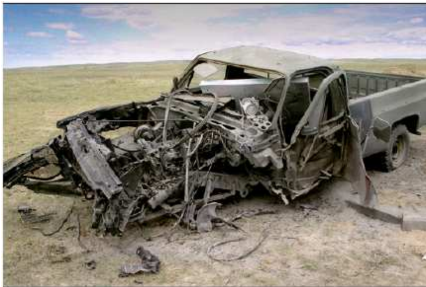
Figure 1.2: Unprotected 5/4 Truck After Mine Test [1]
