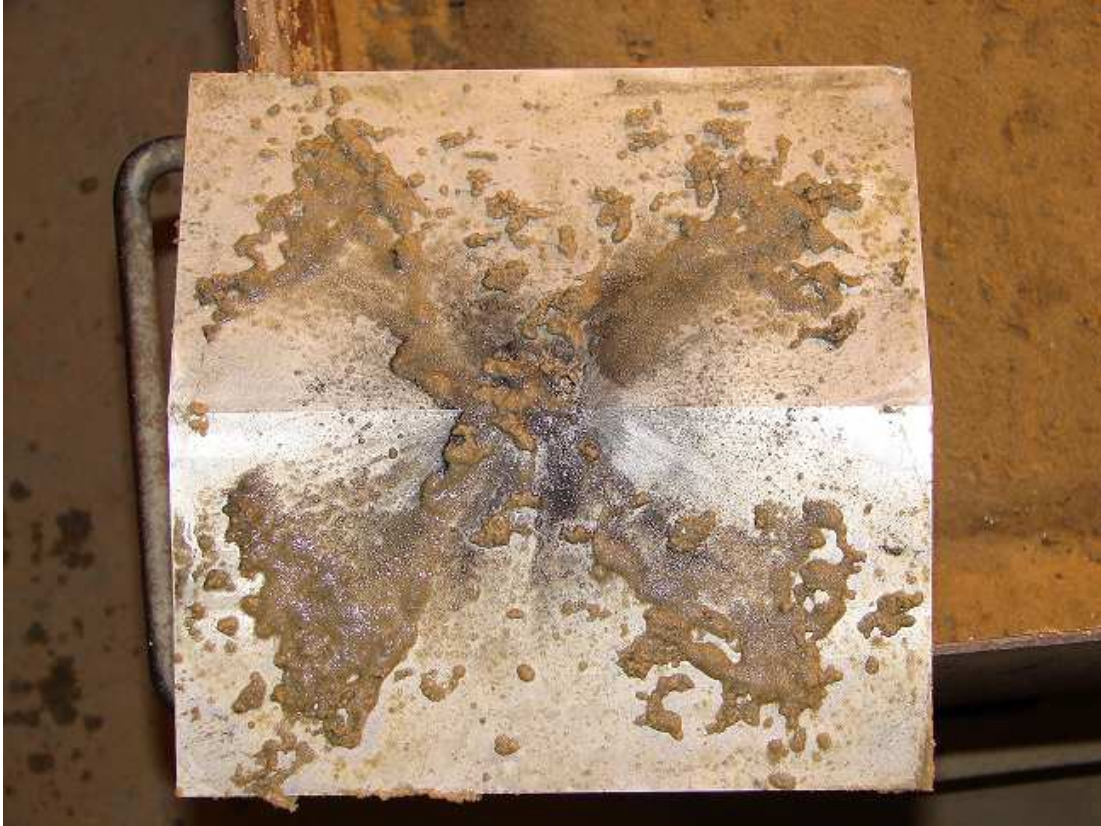
Figure 4.33: Spray Pattern on the Underside of the 13° Plate
