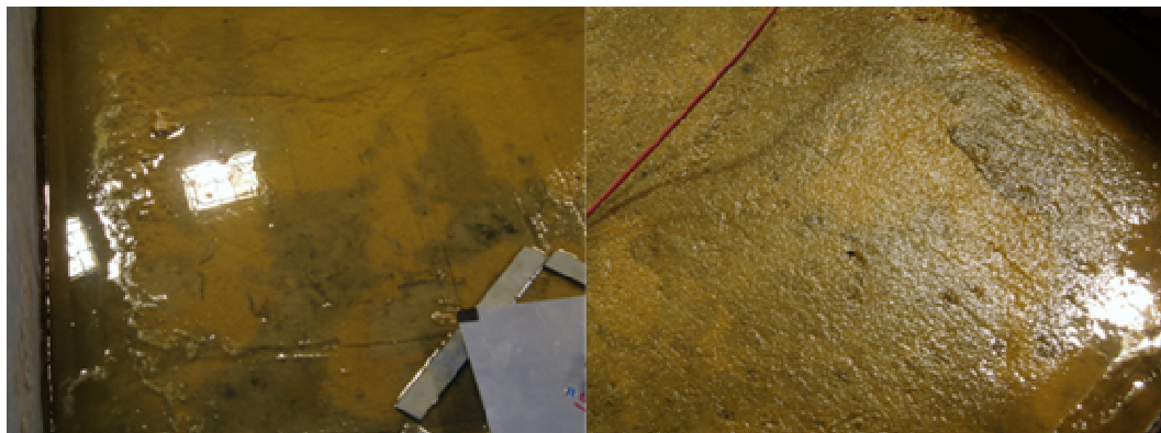
Figure 3.22: Oversaturated Sand (Left) and Properly Saturated Sand (Right)
