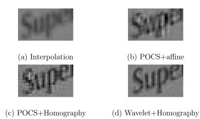
Figure 5.6: Comparison of one reconstructed HR region for various methods.
