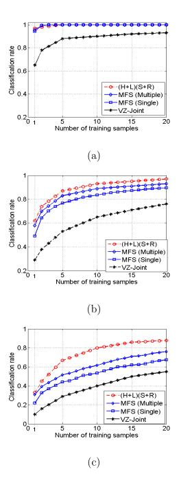
Figure 4.17: Classification rate vs. number of training samples. Three methods are compared: the MFS method, the (H+L)(S+R) method in [3] and the VZ-Joint method in [4]. (a) Classification rate for the best class. (b) Mean classification rate for all 25 classes. (c) Classification rate for the worst class.
