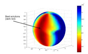
Figure 3.3: The motion valley is the area of smallest values on the error surface in the 2D space of translational directions. The error is found by computing for each translation the optimal rotation.
