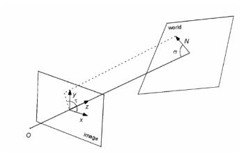
Figure 2.4: The slant of a surface is the angle  $\sigma$  between the negative z-axis and the surface normal, the tilt  $\tau$  is the angle between the projection of the surface normal onto the image plane and the x-axis.
