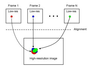
Figure 5.1: Illustration of super-resolution imaging.
