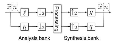
Figure 5.2: The two-channel filter bank.
