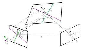
Figure 2.11: A plane with a texture of two orientations  $L_{d_1}$  and  $L_{d_2}$  is imaged under motion.  $\sigma_1$  and  $\sigma_2$  are the angles between the texture lines on the world and the negative z-axis, and  $\tau_1$  and  $\tau_2$  are the angles between the projections of the texture lines on the image plane and the x-axis.
