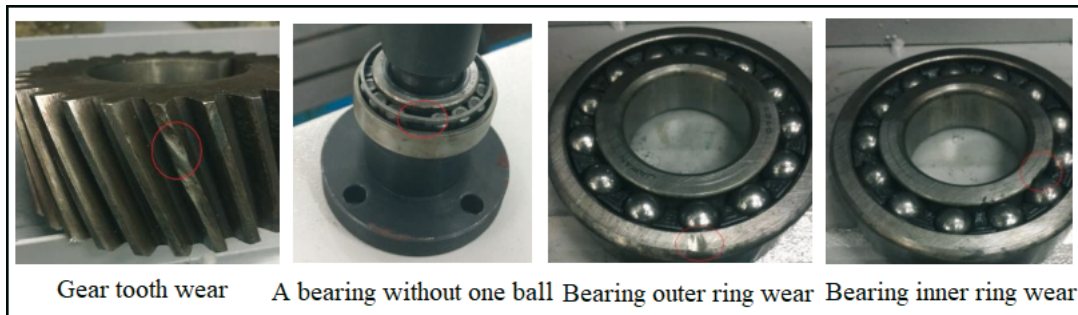
Fig. 5 Gear and bearing faults detected in the gearbox
