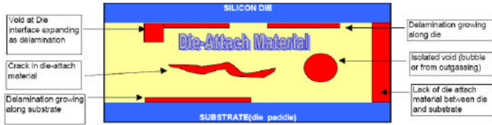
Figure 3.17: Hidden defects revealed by Scanning Acoustic Microscopy
