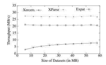
Figure 7.6: Throughput of the pure parsers
