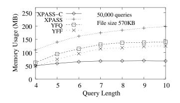
Figure 8.12: Memory Usage for Different Length of Queries
