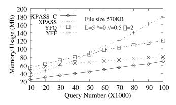
Figure 8.5: Memory Usage for Different Number of Queries
