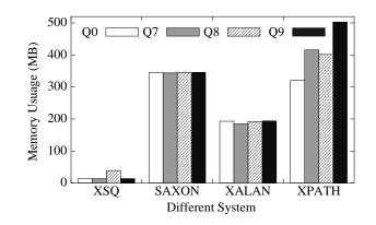
Figure 7.14: Maximum memory allocated for queries over the 58MB dataset
