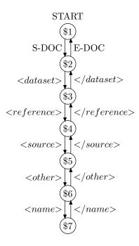
Figure 4.33: HPDT generated for query /dataset/reference/source/other/name
