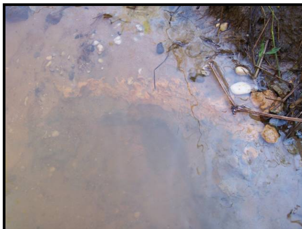
Figure 30. Photo of sulfidic materials under the Manokin Branch west of DX5 at UMES.
