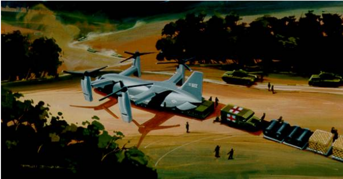
Figure 1.3: Proposed design of the Quad Tilt Rotor (QTR) [3].
