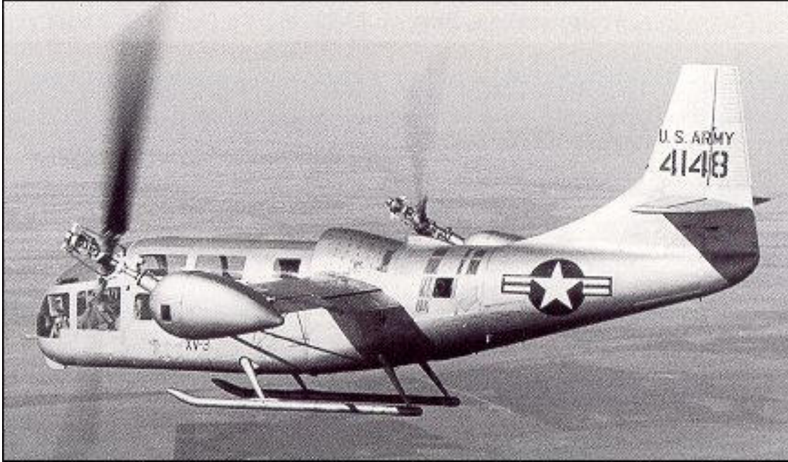
Figure 1.2: Picture of first tilt rotor, XV-3, in forward flight [2].
