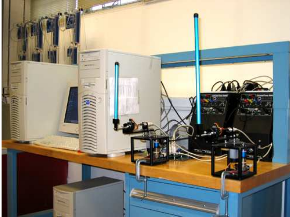
Figure 7.4: Experiment 1: Stabilizing two rotary inverted pendulums at their unstable equilibria.
