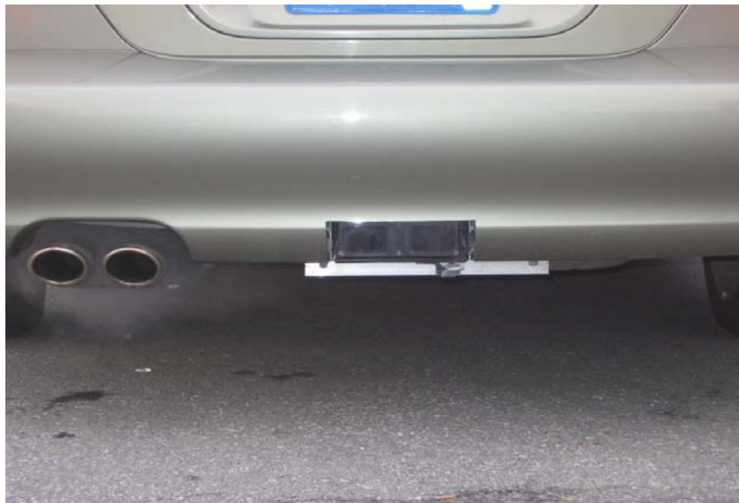
Figure 3. Infrared sensor mounted on the back bumper of the test vehicle
