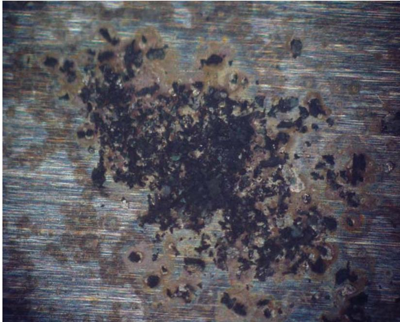
Figure 5.10: Deposit of corrosion product on Ni/Pd/Au plated copper coupon after 15-day 85°C/85% RH exposure
