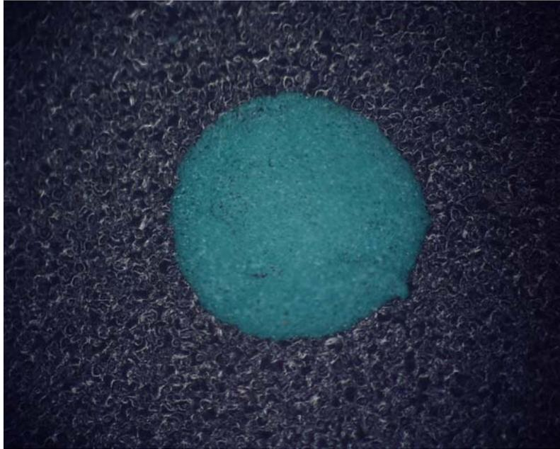
Figure 5.8: Deposit of  $\text{CuCl}_2$  on mold compound surface after 15-day  $85^\circ\text{C}/85\% \text{RH}$  exposure
