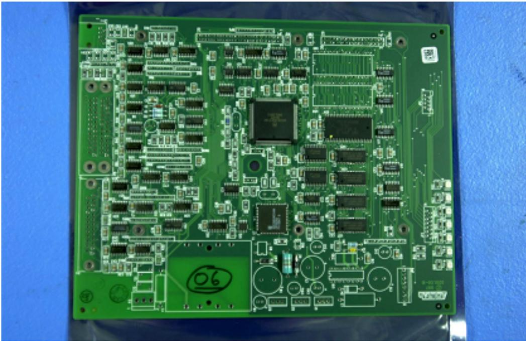
Figure 3.5: Test board with mounted components from Telcordia
