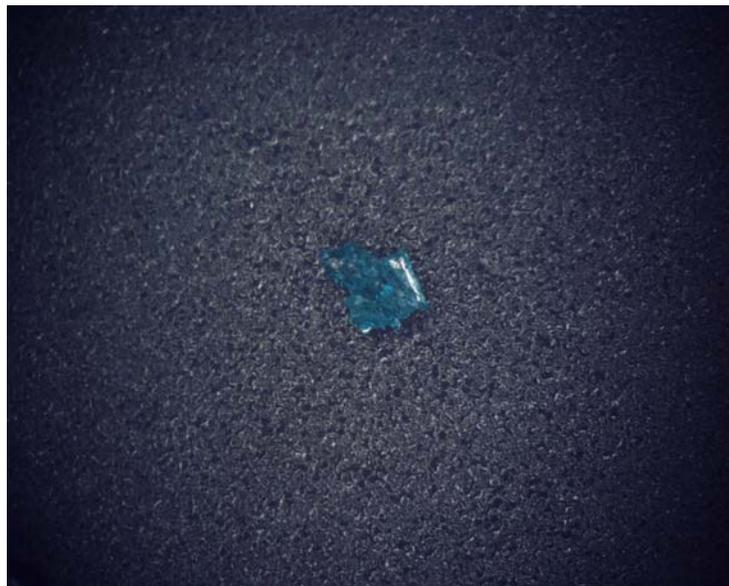
Figure 5.7: Deposit of  $\text{CuCl}_2$  on mold compound surface before  $85^\circ\text{C}/85\%$  RH exposure
