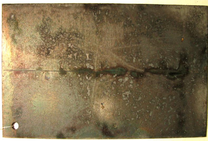
Figure 3.28 Corrosion on sample B after 10-day Telcordia Outdoor MFG test
