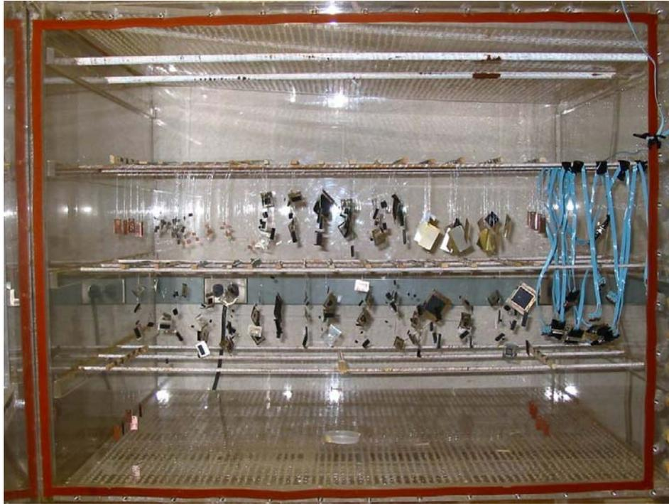
Figure 2.3 Test samples set-up for a MFG test during the study
