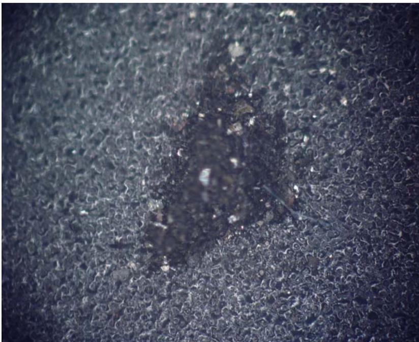
Figure 5.11: Deposit of corrosion product on mold compound before exposure
