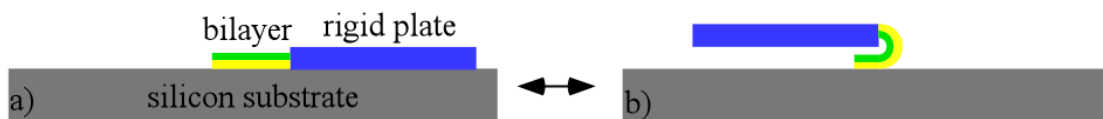
Figure 7. Schematic of a bilayer microactuator. a) The bilayer was fabricated on top of a silicon substrate. A rigid plate was connected to the bilayer. b) When voltages were applied, PPy changed volume; the bilayer bent to actuate the rigid plate. (Courtesy of Smela.)
