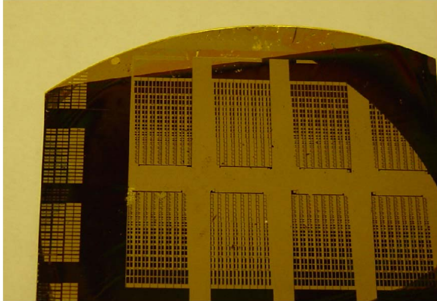
Figure 78. Overview of the sample for bending measurement. There are around 3,000 bilayers on a wafer quarter. All the bilayers have the same PPy: Au thickness ratio, but different bilayer dimensions. (Courtesy of Christophersen.)
