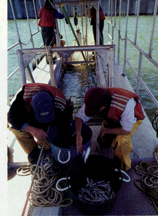
During a test run, water gushing to the surface carries fish from the lower reservoir to be collected with a recovery net, then sorted and counted. Excessive numbers of fish — 88,000 in just over an hour — passed through the turbines in the spring of 1993, halting daytime tests.
