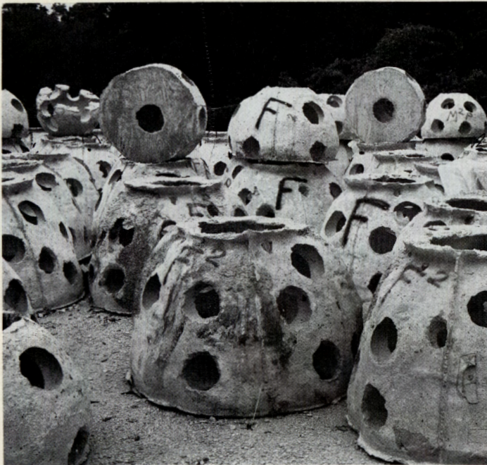
Ready for deployment to a coastal fishing site, concrete spheres known as reef balls attract fish by providing hives of hideouts on an otherwise featureless sea floor.
