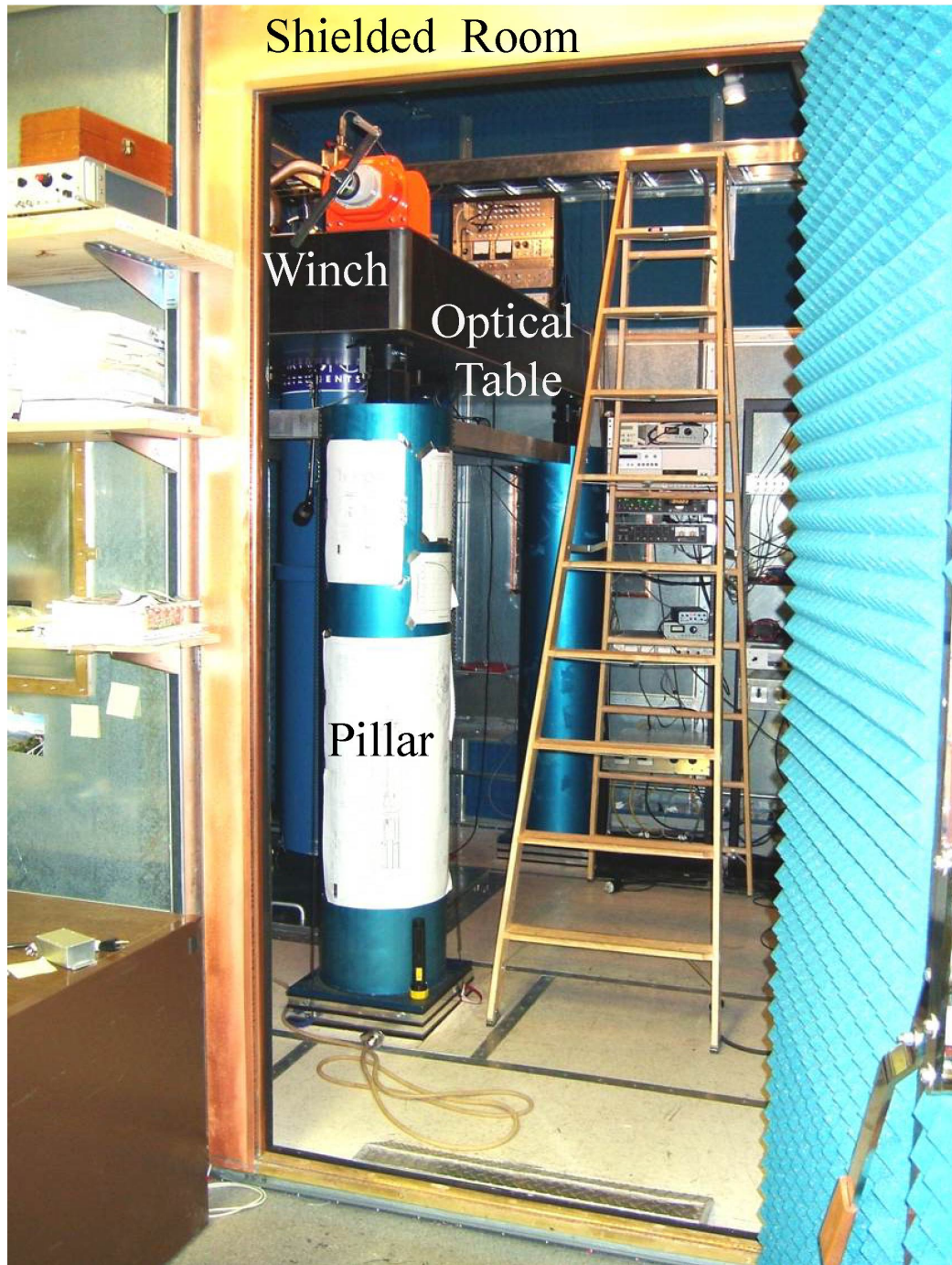
Figure 4.4: Picture of shielded room and optical table. The ^4\text{He} dewar is visible behind the front pillar. A winch is used to raise the dewar over the refrigerator.
