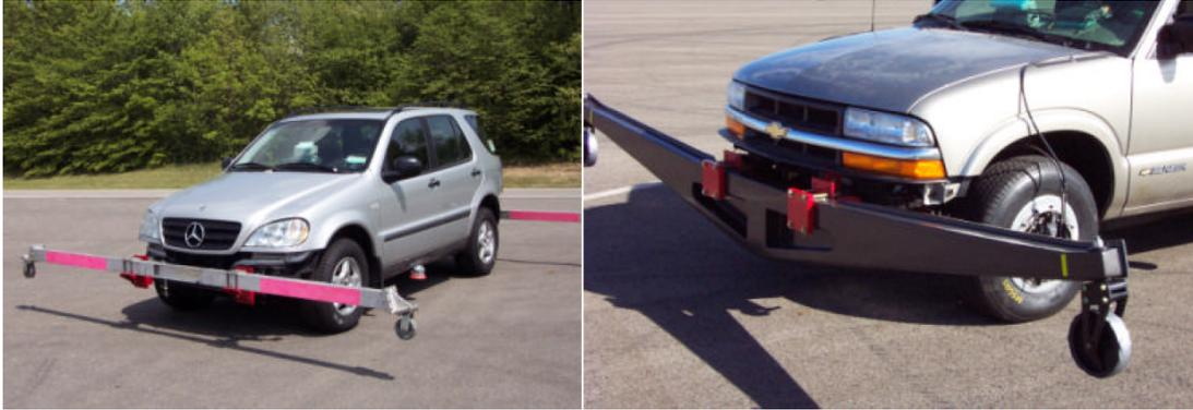
Figure 1.1: Aluminum and Carbon Fiber Outriggers used by NHTSA [7]
