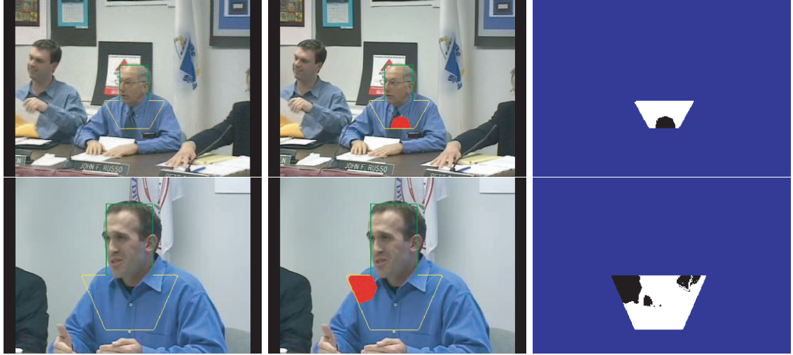
Figure 4.1: Detection of outliers. The image in the first column is the model image. Second column images are used as instances. To synthesize outliers, a 15% size block with red color pixels is created. In the third column the inliers and outliers are shown as white and black points, respectively.
