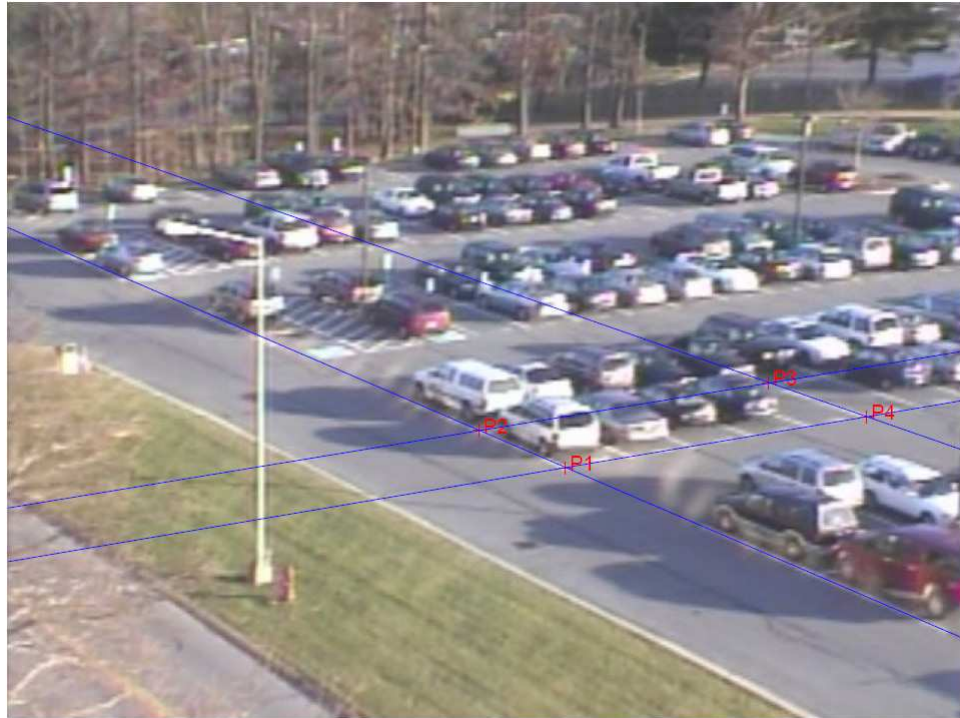
Figure 4.5: The original frame used in the affine recovery process, showing the two pairs of parallel lines used to locate the vanishing line.
