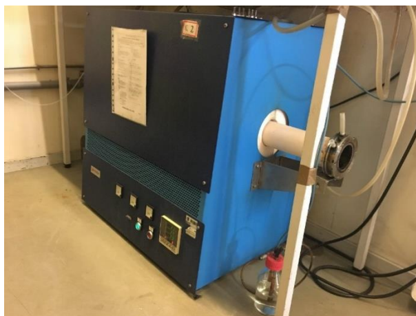
Figure A.2. Alumina tube inside a tubular horizontal Termolab TH furnace.
