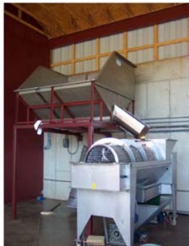
Figure 4: External destemming and crushing equipment at Barbourville
