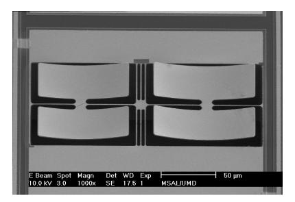
Figure 5.14: Micrograph of a mechanical-amplifier actuator cooled down to 30 K. The blades curl up due to the mismatch of CTEs among silicon nitride, chromium, and gold layers.
