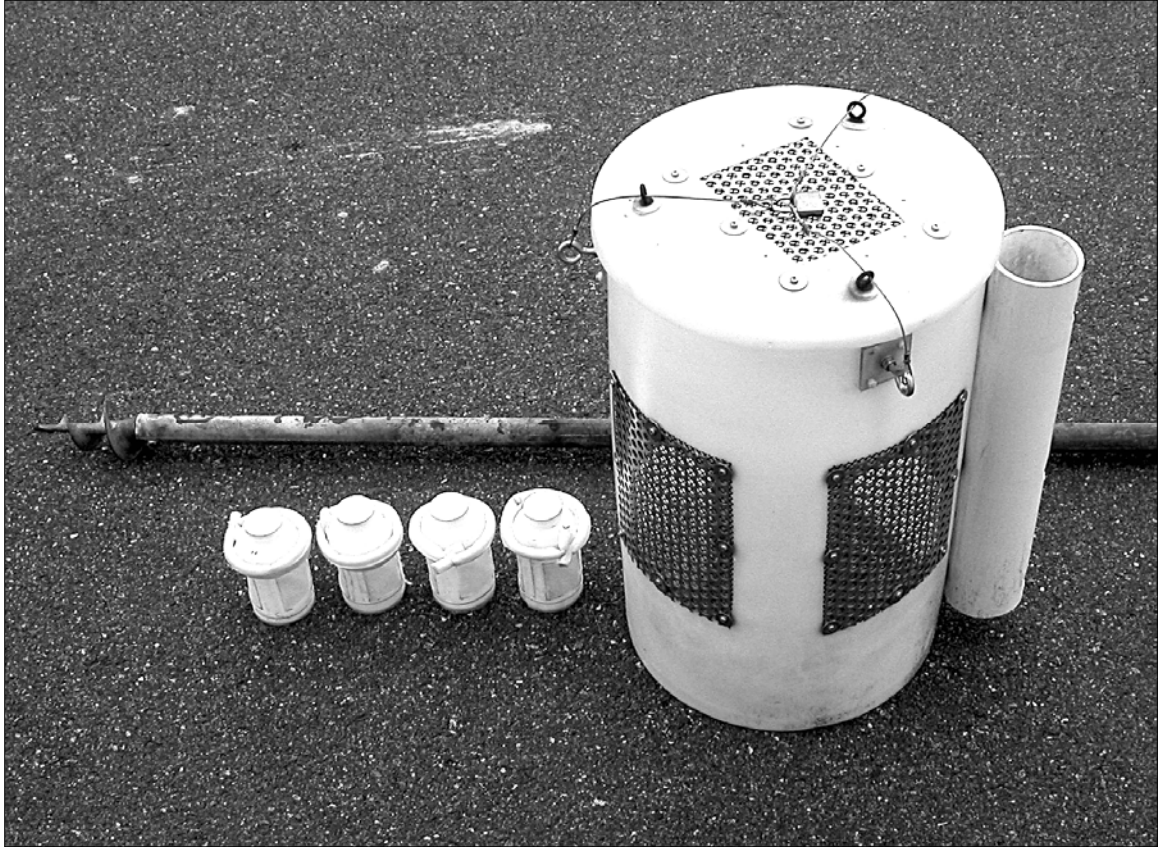
Figure 22. Detail of fish caging apparatus including protective barrel, floating baskets, and galvanized mounting post.
