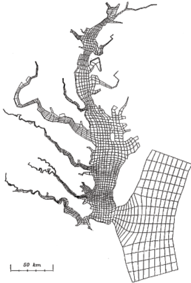
Fig. 2.4 Boundary fitted grid of the Chesapeake Bay hydrodynamic model.
