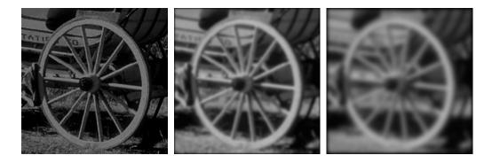
Figure 1.1: Gaussian smoothing, left: original image; middle:  $\sigma = 2$ ; right:  $\sigma = 4$ .
