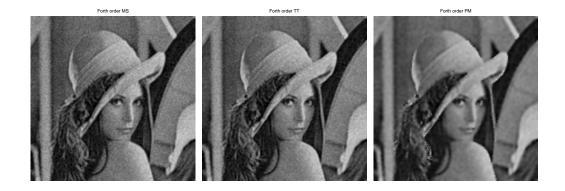
Figure 6.15: Fourth order PDE smoothing results for k = 1 at t = 500, from left to right, Minimal surface, Tumblin-Turk, You-Kaveh diffusion function.
