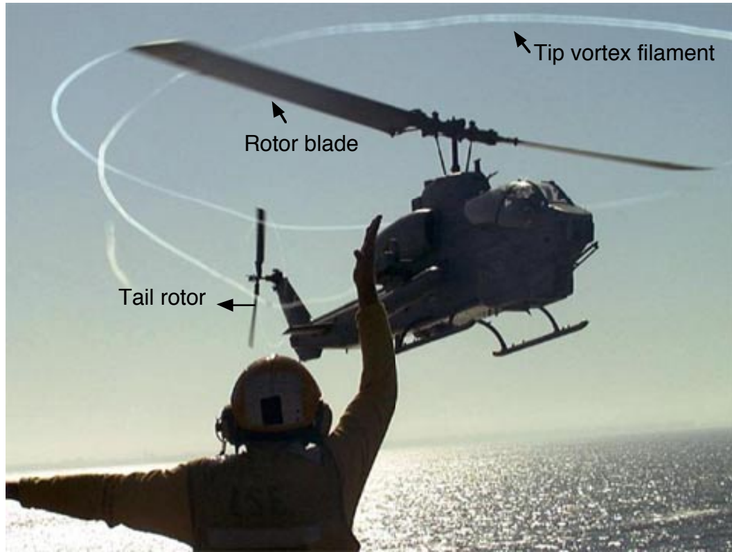
Figure 1.1: Photograph of tip vortices trailing the rotor blades of the Bell AH-1 Cobra. (Courtesy of the US Navy.)
