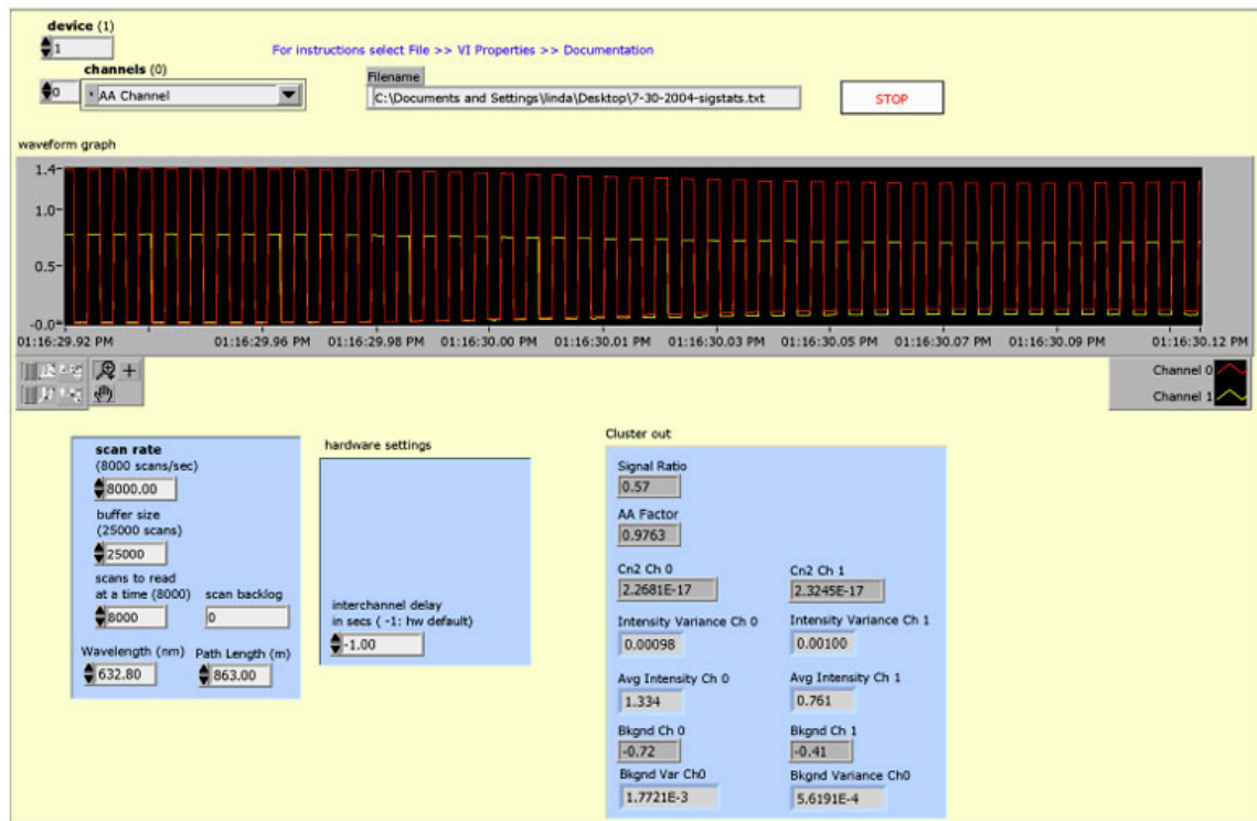
Fig. 3.7: Front panel of the LabVIEW program designed to calculate and record irradiance statistics for the aperture averaging experiment.
