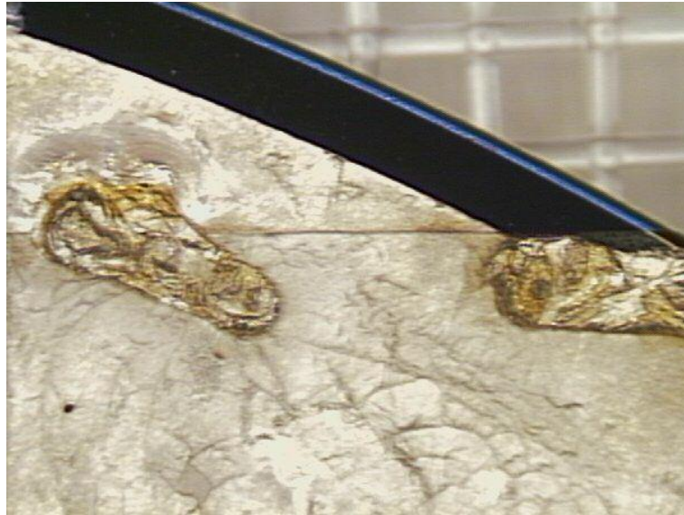
Figure 3-4: Oxide bag after complete reflow
