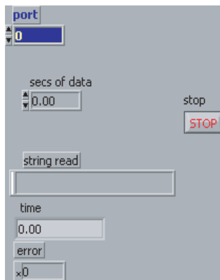
Figure B.10: Front panel of Labview program (stod0061704.vi) used to acquire the serial digital data coming from the measurement probes on the rotating assembly.
