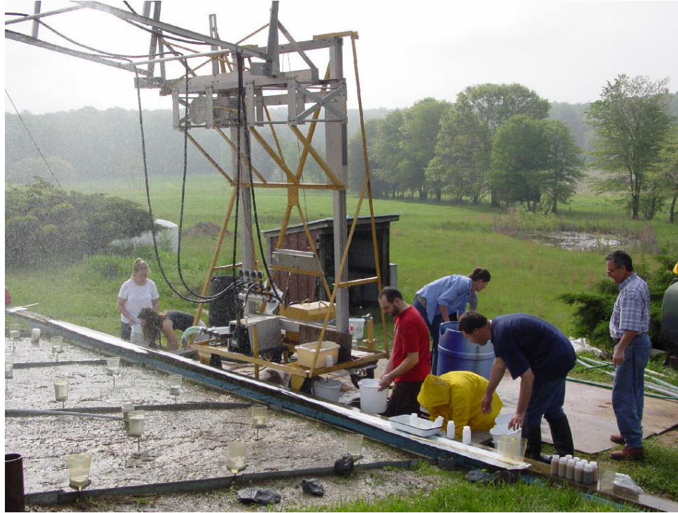
Figure 2.13. Rainfall simulator used to generate rain for experiments
