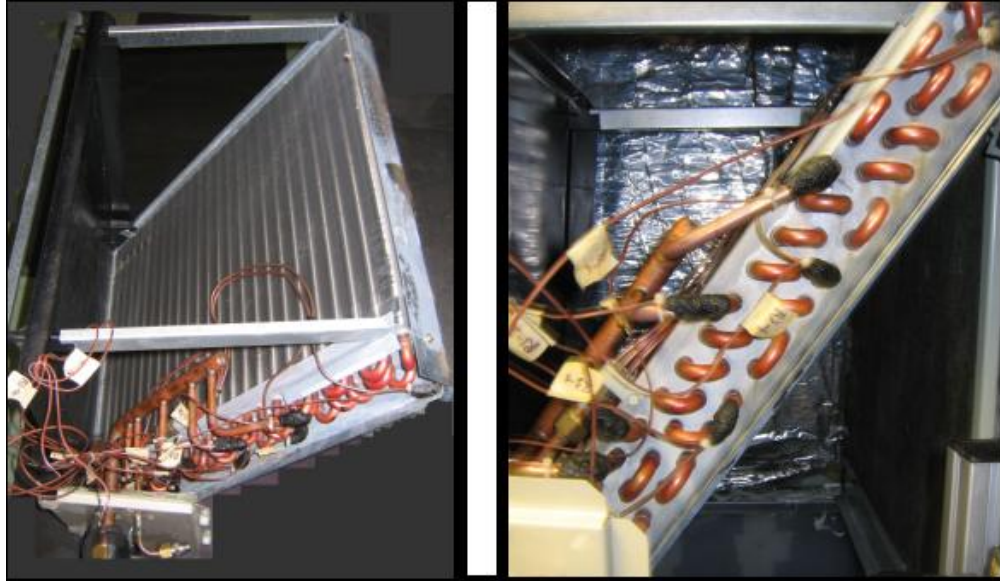
Figure 4.3: Slope Coil Heat Exchanger used as Evaporator in the Oil Retention Test
