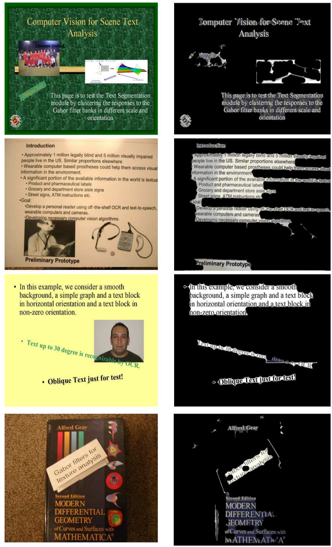
Figure 3.7: In this example, we test the power of text segmentation algorithm for different presentation/poster and outdoor scene text layout. From top-down images are (a)-(d). (a) and (c) are presentation slides with different text size and orientation, different graphs and complex or simple background. (c) is an image of a poster with simple background. (d) is an image of a book on the textured background. The results of text segmentation are shown in the second column.
