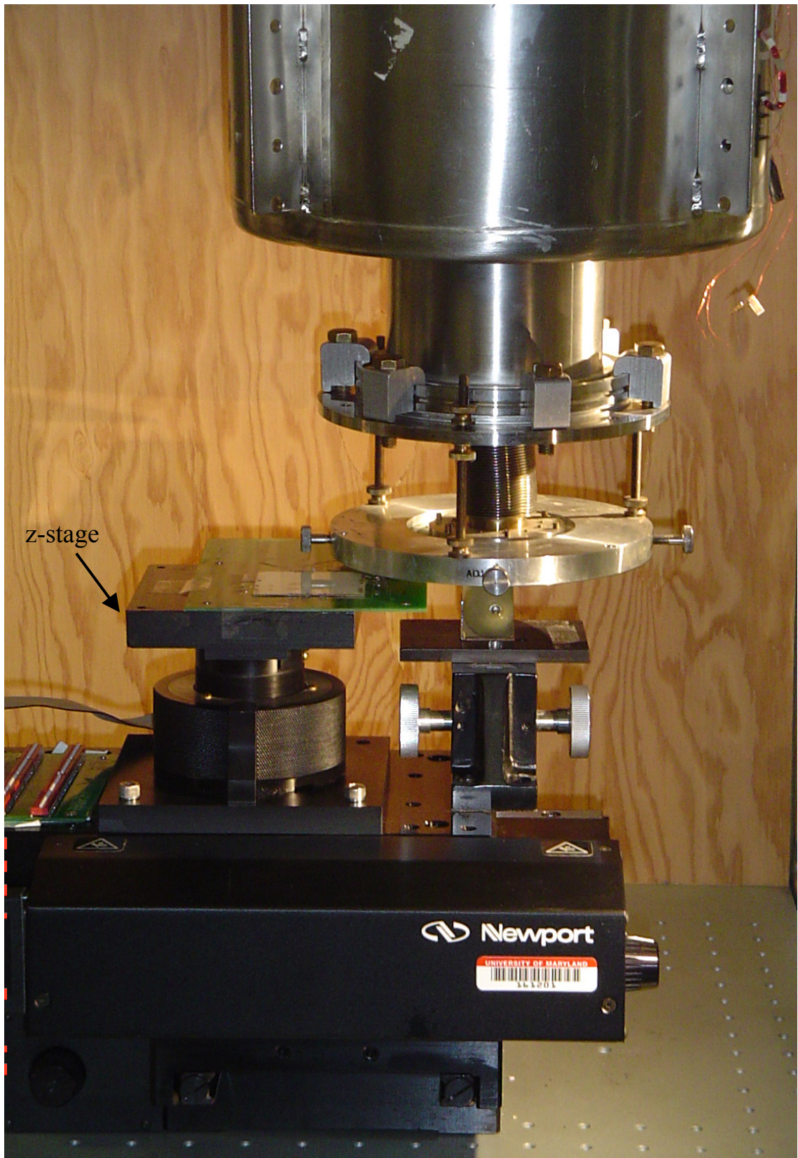
Figure 6.10: Photograph of multi-channel SQUID system with the new stage.
