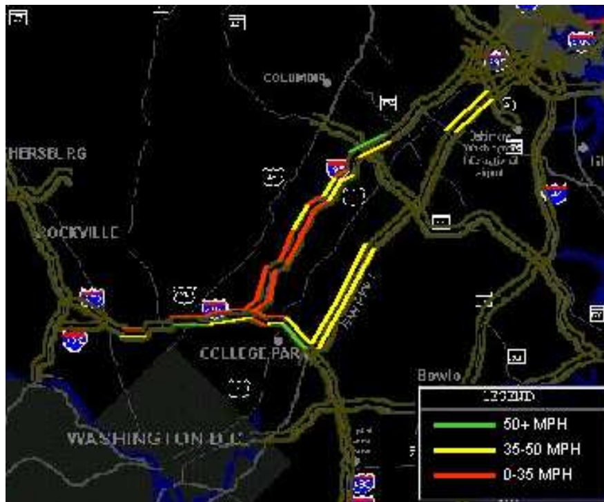
Figure 10. Comparative display showing only the areas where the traffic is worse than usual. The color-coding remains the same, showing absolute speeds.
