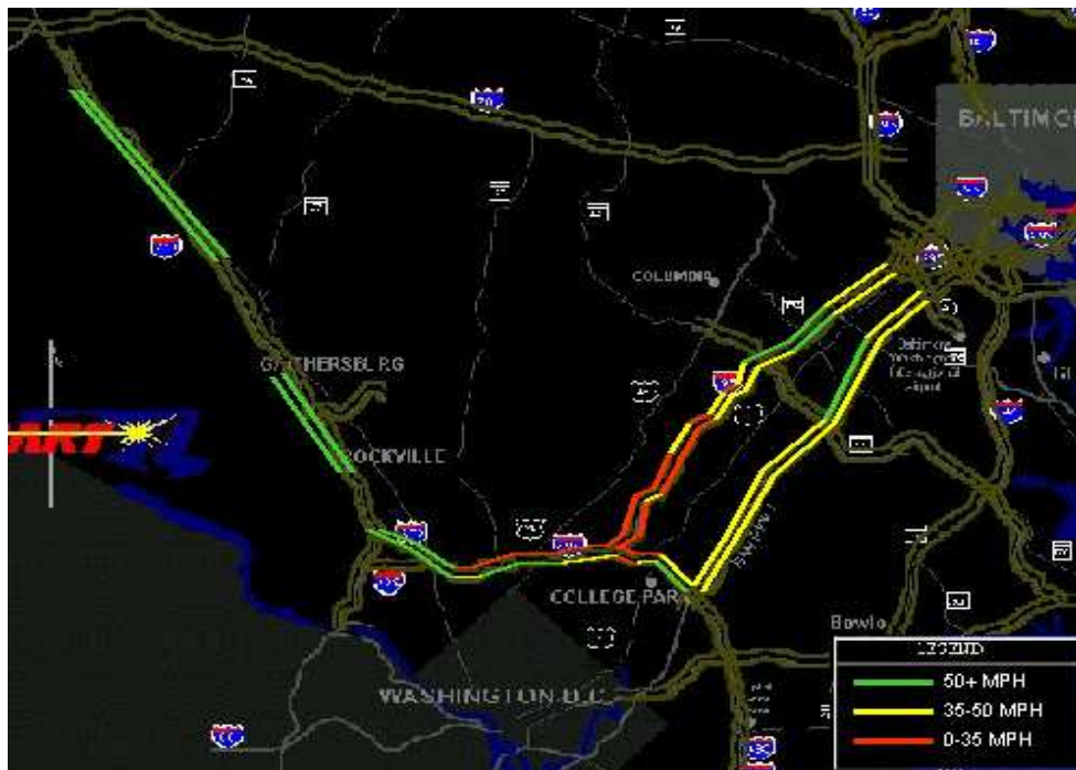
Figure 6. Segment Display. Only a section of limited length is extrapolated from a sensor data point. Therefore the coverage is not complete in areas where there are fewer sensors available.
