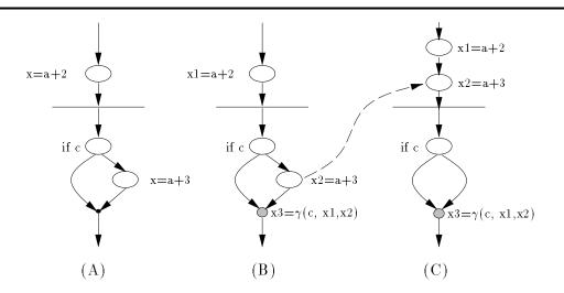
Figure 5.6: Speculative Code Motion: (A) Original Code, (B) Corresponding GSA Code and (C) Speculatively Transformed Code
