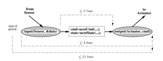
Figure 1.2: Event-Based Specification of Sensor-Controller System
