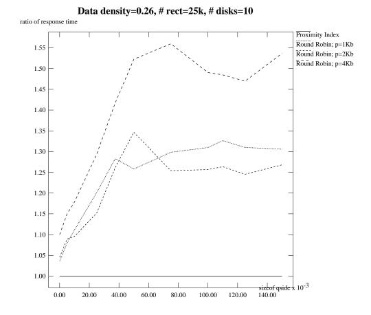
Figure 3.15: Relative response time (RR over PI) vs. query size for different page sizes.
