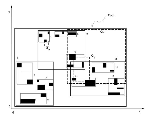
Figure 3.1: Data (dark rectangles) organized in an R-tree. Fanout=3. Dotted rectangles indicate queries.
