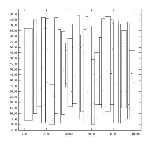
Figure 4.2: MBR of nodes generated by the 'lowx packed R-tree' algorithm.
