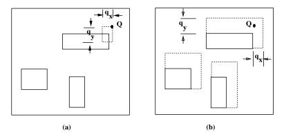
Figure 4.8: (a) Original nodes along with rectangular query  $q_x \times q_y$ ; (b) Extended nodes with point query Q.
