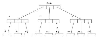
Figure 2.2: The file structure for the R-tree in Figure 2.1 (fanout=3).
