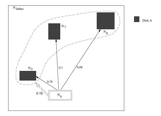
Figure 3.9: The proximity index between the node  $N_0$  and the set  $\{N_5, N_7, N_8\}$ . The numbers next to the solid arrows show the proximity measure.
