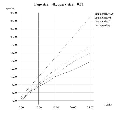
Figure 3.21: Speed-up of the Multiplexed R-tree vs. number of disks with query size = 0.25.
