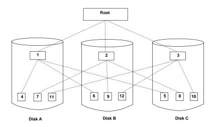
Figure 3.2: An R-tree stored on three disks.
