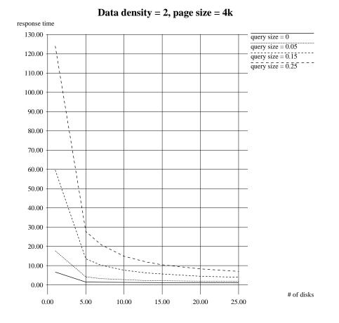
Figure 3.20: Response time of the Multiplexed R-tree vs. number of disks for different query sizes.
