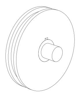
Figure 3: Shaft and Pulley Assembly.
