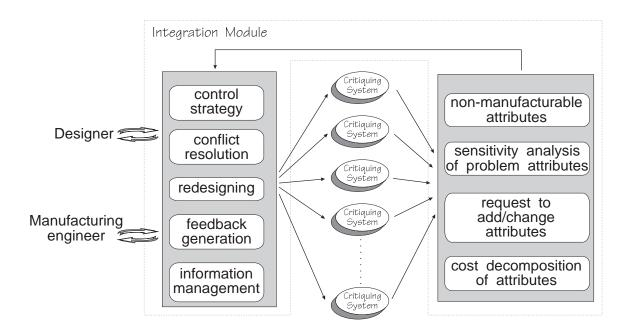
Figure 10: Integrating the operation of multiple critiquing systems.
