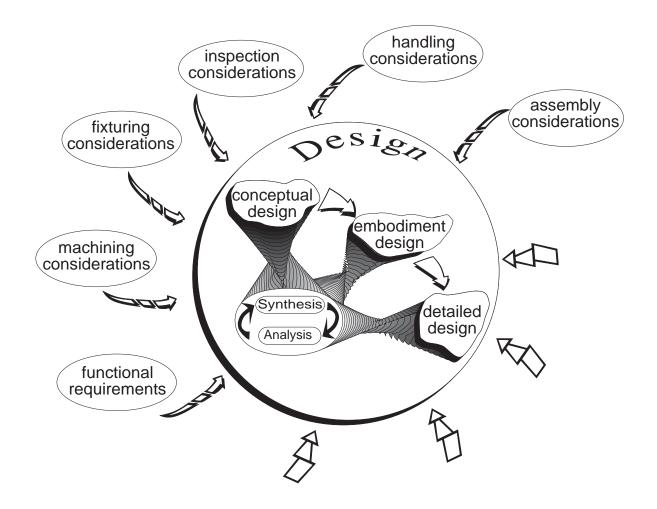
Figure 2: Design For Manufacturability.
