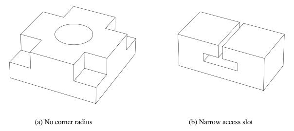
Figure 8: Design posing problem for machining.
